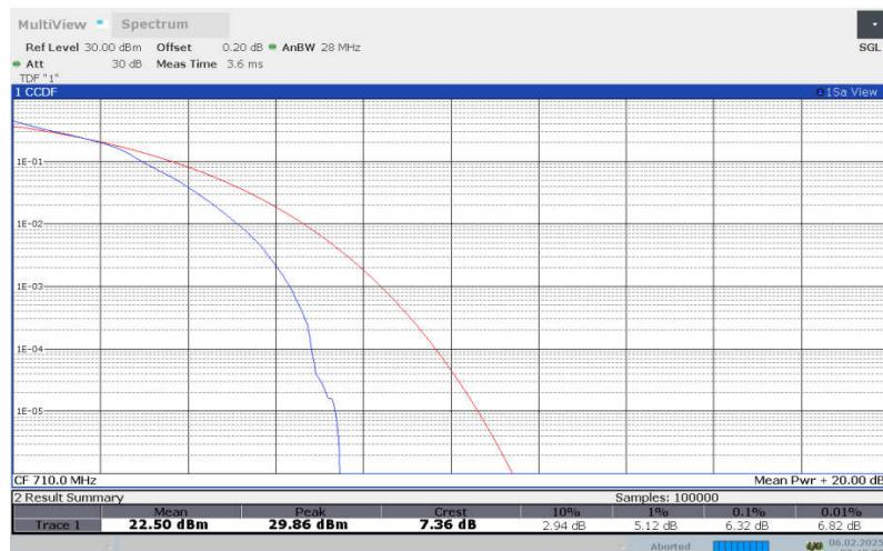
**LTE Band 17, 10MHz Bandwidth, 64QAM**
