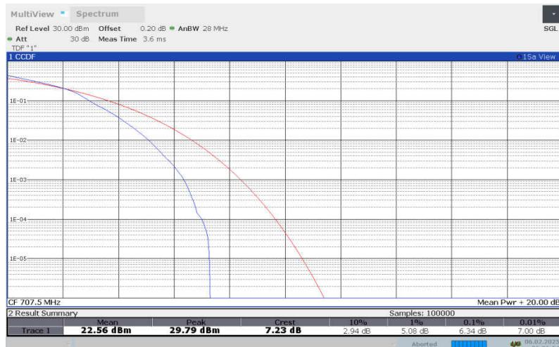
**LTE Band 12 , 3MHz Bandwidth,64QAM**
