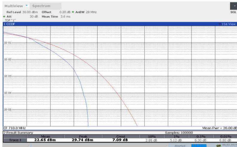
**LTE Band 17 , 5MHz Bandwidth,64QAM**
