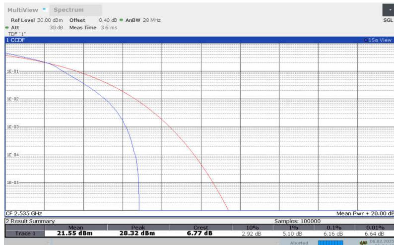
**LTE Band 7, 5MHz Bandwidth, 64QAM**
