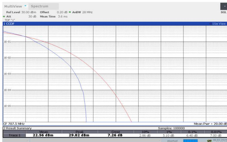
**LTE Band 12 , 5MHz Bandwidth,64QAM**
