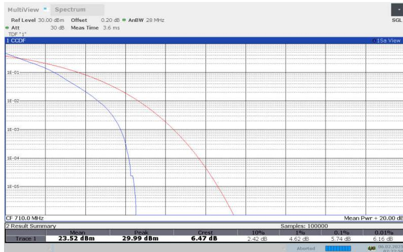
**LTE Band 17 , 5MHz Bandwidth,16QAM**
