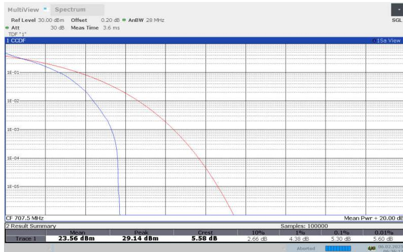
**LTE Band 12 , 1.4MHz Bandwidth,16QAM**
