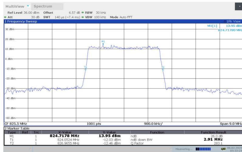
**LTE Band 26 , 3MHz Bandwidth,LOW,64QAM (-26dBc OBW)**
