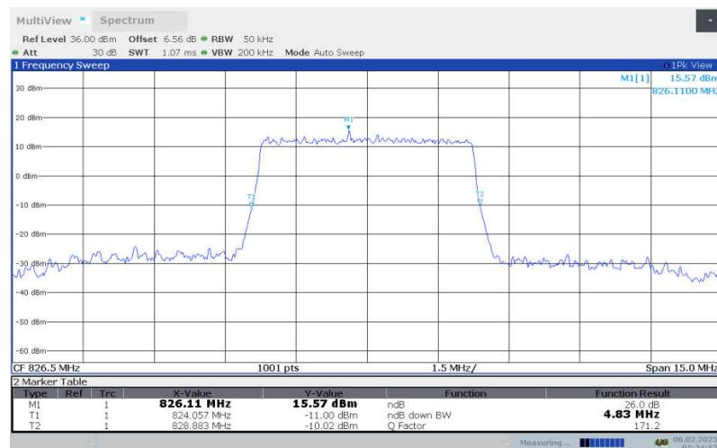
**LTE Band 26 , 5MHz Bandwidth,LOW,64QAM (-26dBc OBW)**
