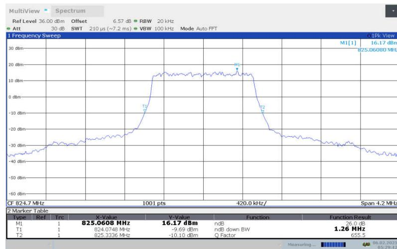
**LTE Band 26 , 1.4MHz Bandwidth,LOW,16QAM (-26dBc OBW)**
