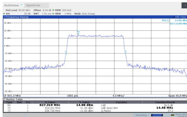
**LTE Band 26 , 15MHz Bandwidth,LOW,64QAM (-26dBc OBW)**
