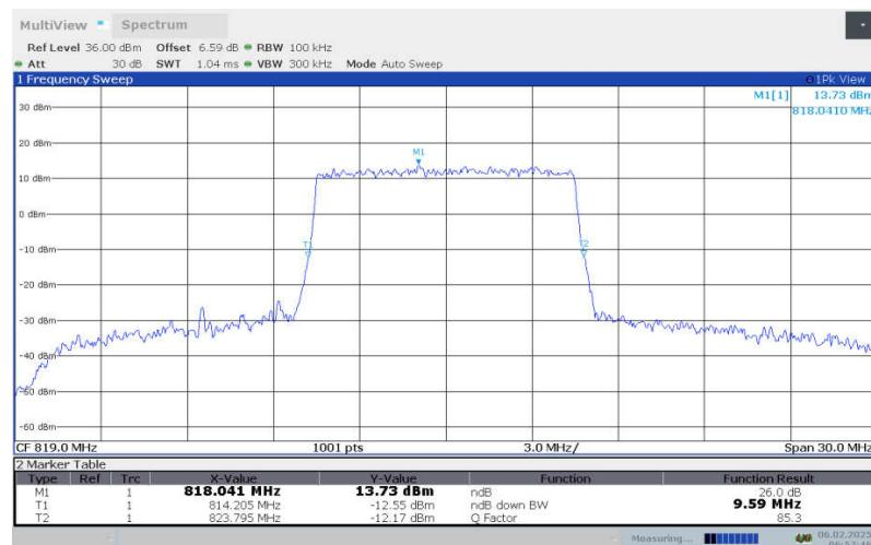
**LTE Band 26 , 10MHz Bandwidth,LOW,64QAM (-26dBc OBW)**
