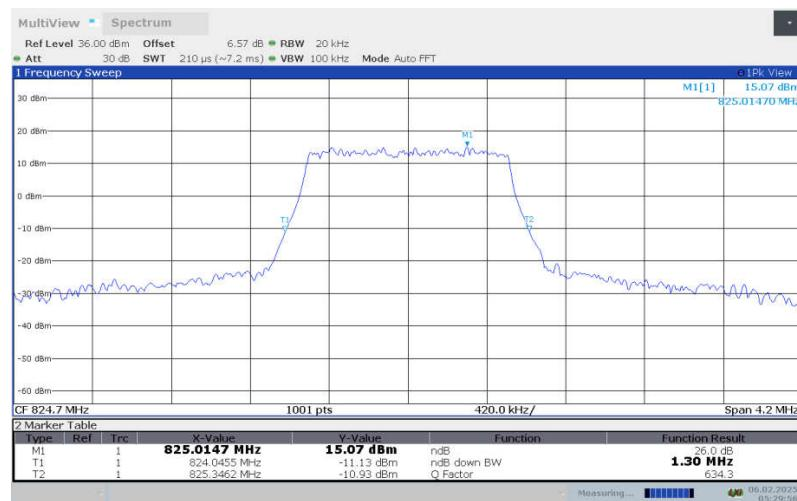
**LTE Band 26 , 1.4MHz Bandwidth,LOW,64QAM (-26dBc OBW)**
