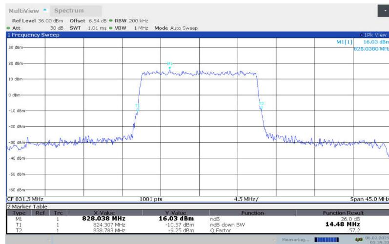
**LTE Band 26 , 15MHz Bandwidth,LOW,16QAM (-26dBc OBW)**
