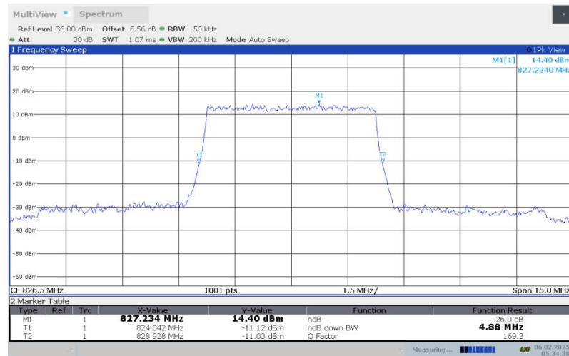
**LTE Band 26 , 5MHz Bandwidth,LOW,16QAM (-26dBc OBW)**
