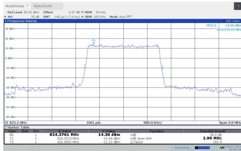
**LTE Band 26 , 3MHz Bandwidth,LOW,16QAM (-26dBc OBW)**
