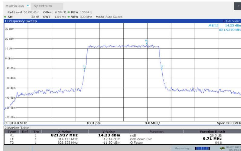
**LTE Band 26 , 10MHz Bandwidth,LOW,16QAM (-26dBc OBW)**
