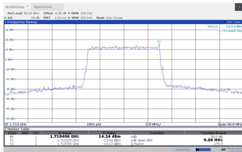
**LTE Band 4 , 10MHz Bandwidth,LOW,64QAM (-26dBc OBW)**
