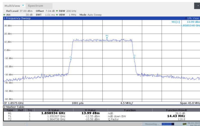
**LTE Band 2 , 15MHz Bandwidth,LOW,64QAM (-26dBc OBW)**
