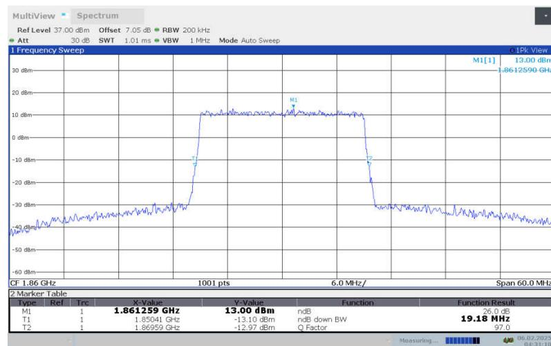
**LTE Band 2 , 20MHz Bandwidth,LOW,64QAM (-26dBc OBW)**
