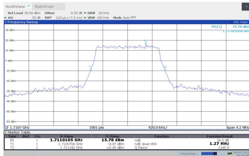
**LTE Band 4, 1.4MHz Bandwidth,LOW,64QAM (-26dBc OBW)**
