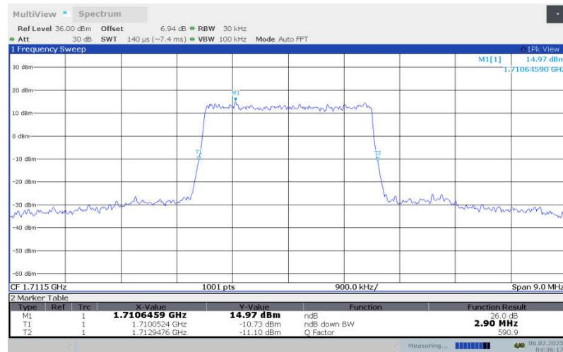
**LTE Band 4, 3MHz Bandwidth,LOW,16QAM (-26dBc OBW)**
