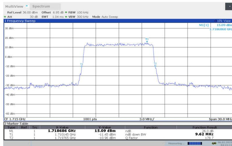
**LTE Band 4 , 10MHz Bandwidth,LOW,16QAM (-26dBc OBW)**
