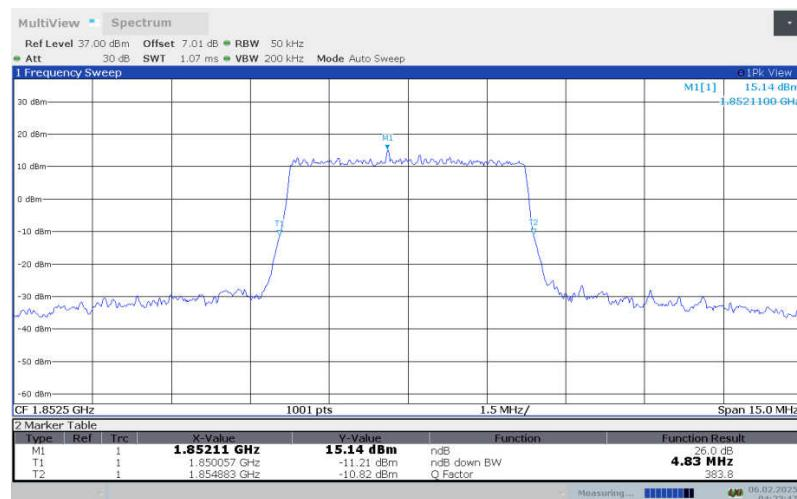
**LTE Band 2, 5MHz Bandwidth,LOW,64QAM (-26dBc OBW)**
