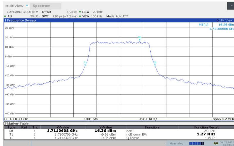
**LTE Band 4, 1.4MHz Bandwidth,LOW,16QAM (-26dBc OBW)**
