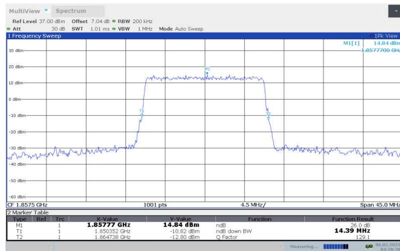
**LTE Band 2 , 15MHz Bandwidth,LOW,16QAM (-26dBc OBW)**
