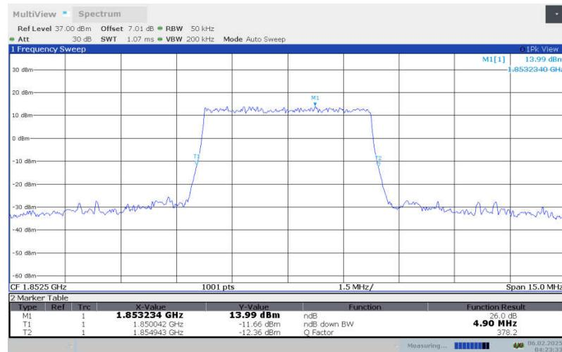
**LTE Band 2, 5MHz Bandwidth,LOW,16QAM (-26dBc OBW)**
