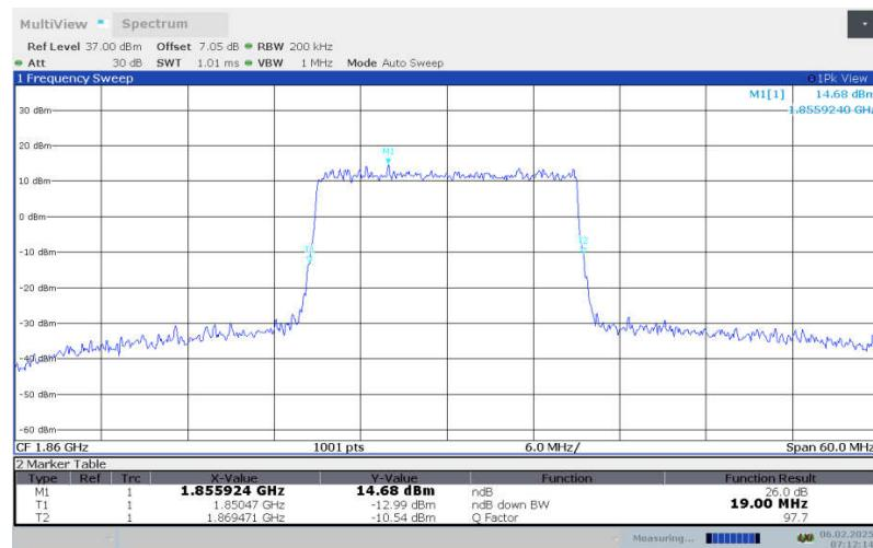
**LTE Band 2 , 20MHz Bandwidth,LOW,16QAM (-26dBc OBW)**
