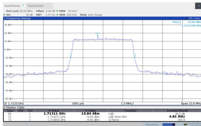
**LTE Band 4, 5MHz Bandwidth,LOW,64QAM (-26dBc OBW)**
