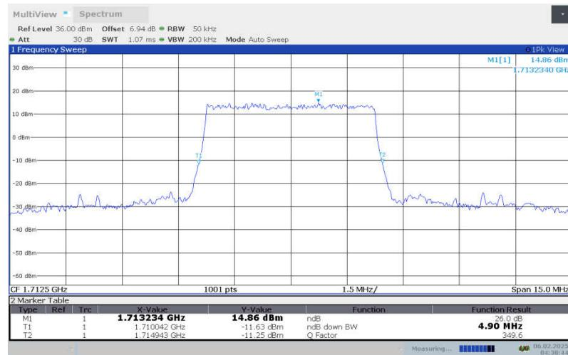
**LTE Band 4, 5MHz Bandwidth,LOW,16QAM (-26dBc OBW)**
