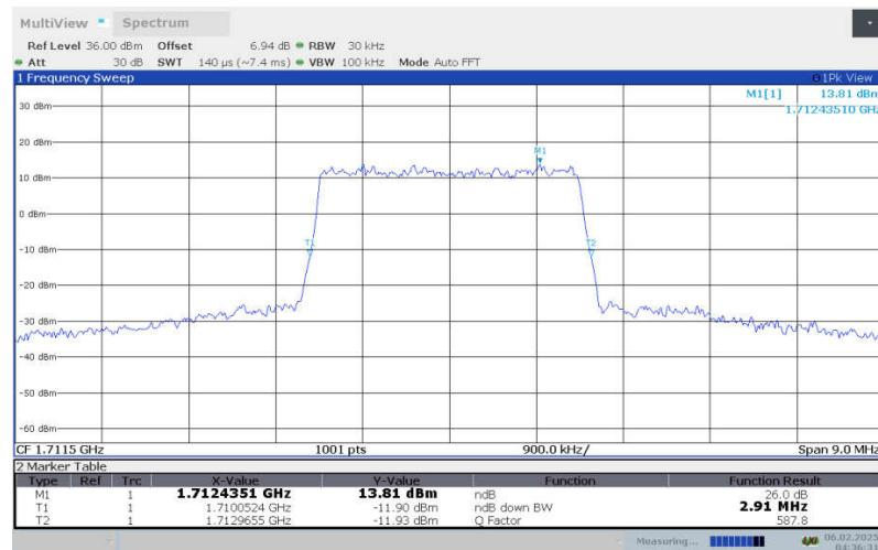
**LTE Band 4, 3MHz Bandwidth,LOW,64QAM (-26dBc OBW)**
