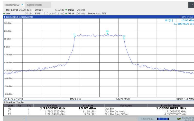
**LTE Band 66 , 1.4MHz Bandwidth,LOW,16QAM (99% OBW)**
