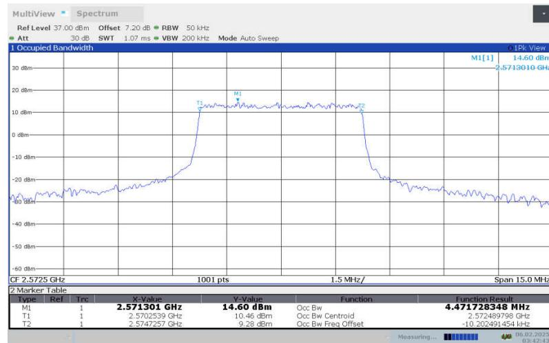
**LTE Band 38 , 5MHz Bandwidth,LOW,16QAM (99% OBW)**
