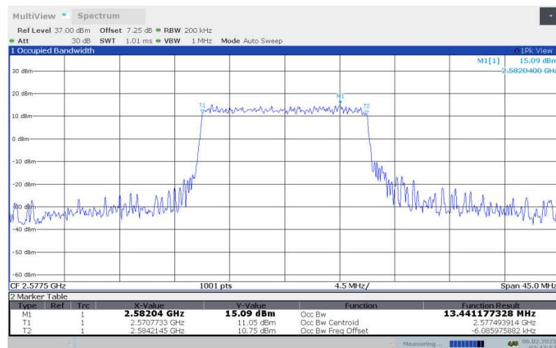
**LTE Band 38 , 15MHz Bandwidth,LOW,64QAM (99% OBW)**
