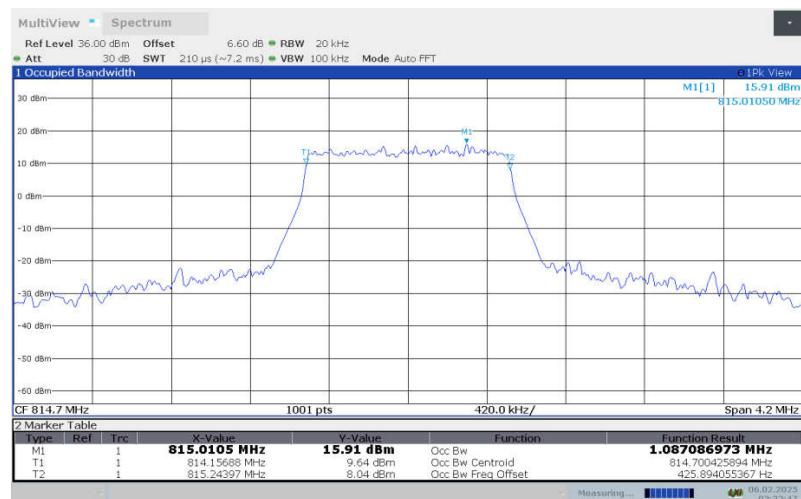
**LTE Band 26 , 1.4MHz Bandwidth,LOW,64QAM (99% OBW)**
