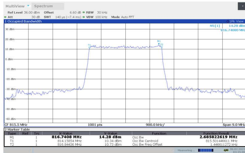
**LTE Band 26 , 3MHz Bandwidth,LOW,16QAM (99% OBW)**
