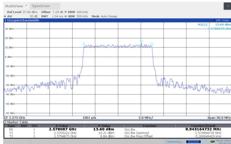
**LTE Band 38 , 10MHz Bandwidth,LOW,64QAM (99% OBW)**
