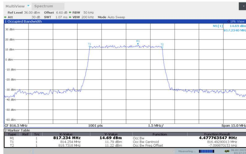
**LTE Band 26 , 5MHz Bandwidth,LOW,16QAM (99% OBW)**
