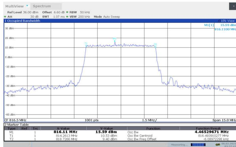
**LTE Band 26 , 5MHz Bandwidth,LOW,64QAM (99% OBW)**
