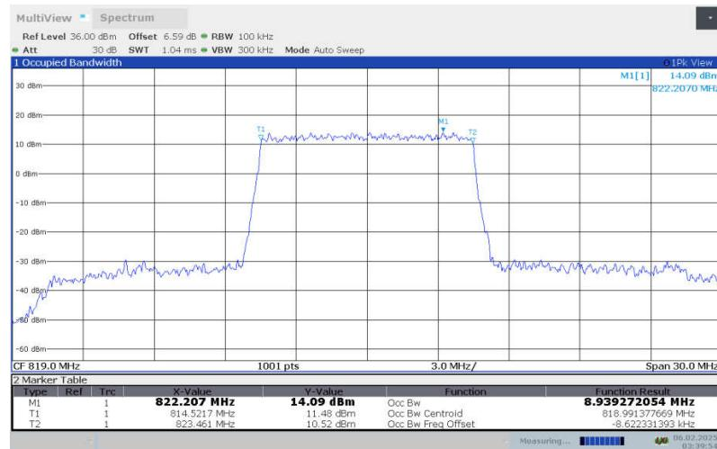
**LTE Band 26 , 10MHz Bandwidth,LOW,16QAM (99% OBW)**
