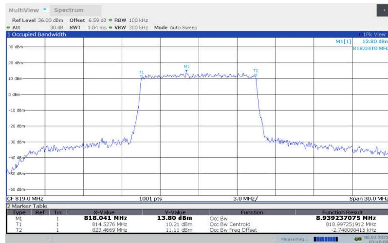
**LTE Band 26 , 10MHz Bandwidth,LOW,64QAM (99% OBW)**
