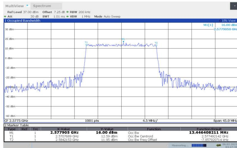
**LTE Band 38 , 15MHz Bandwidth,LOW,16QAM (99% OBW)**
