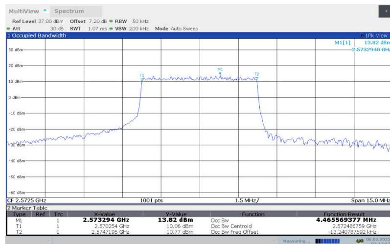
**LTE Band 38 , 5MHz Bandwidth,LOW,64QAM (99% OBW)**
