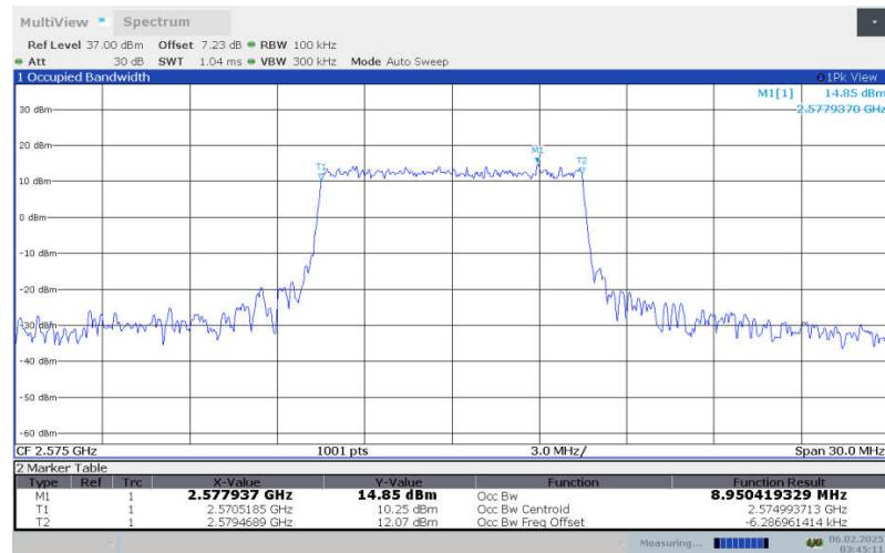
**LTE Band 38 , 10MHz Bandwidth,LOW,16QAM (99% OBW)**
