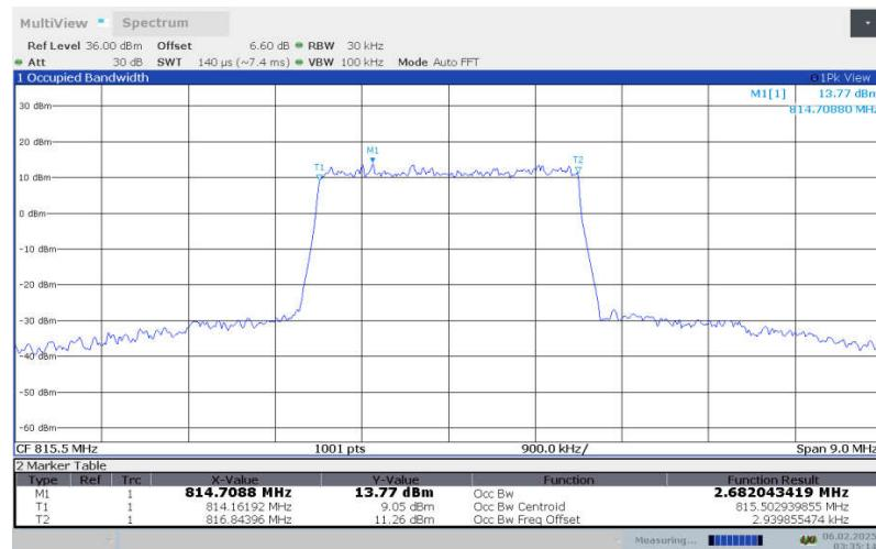
**LTE Band 26 , 3MHz Bandwidth,LOW,64QAM (99% OBW)**
