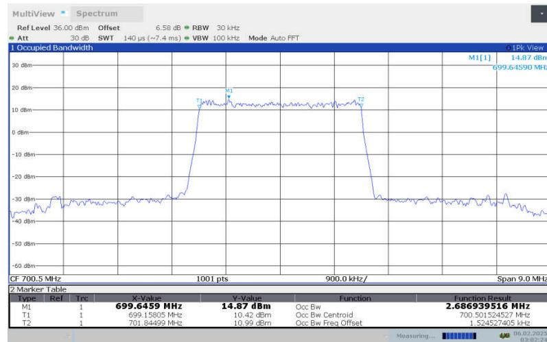
**LTE Band 12 , 3MHz Bandwidth,LOW,16QAM (99% OBW)**
