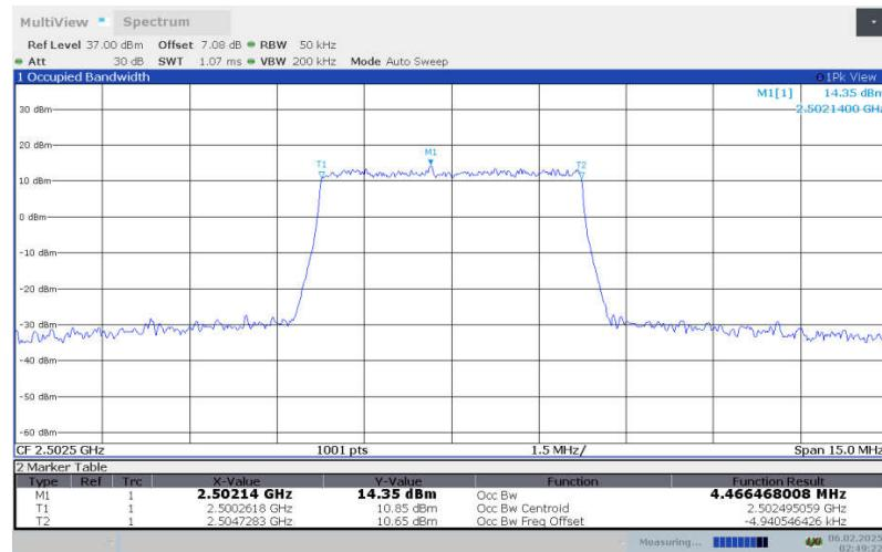
**LTE Band 7 , 5MHz Bandwidth,LOW,16QAM (99% OBW)**
