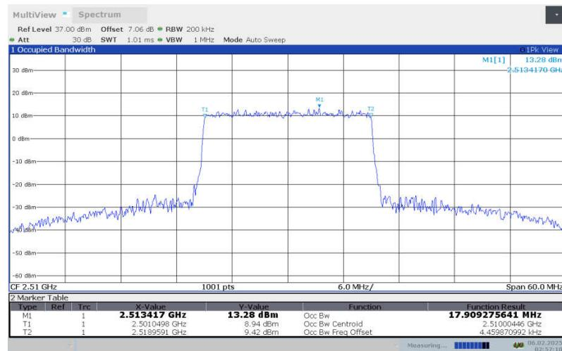
**LTE Band 7 , 20MHz Bandwidth,LOW,64QAM (99% OBW)**
