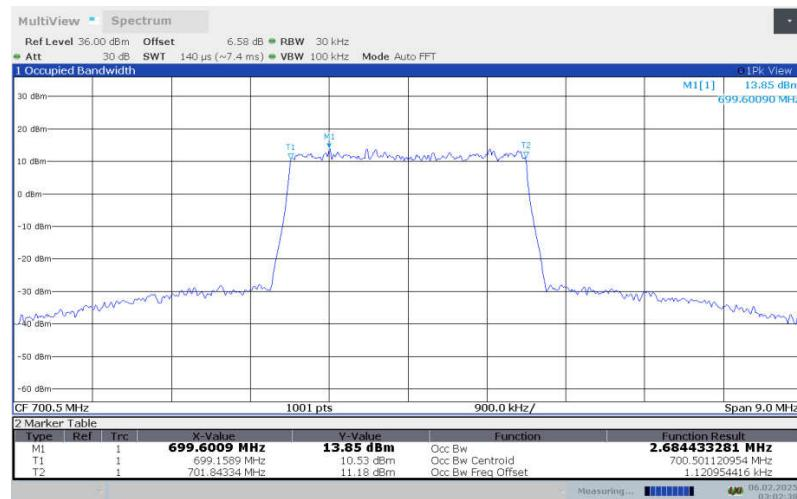
**LTE Band 12 , 3MHz Bandwidth,LOW,64QAM (99% OBW)**
