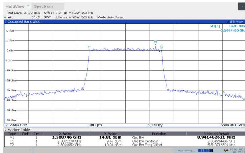
**LTE Band 7 , 10MHz Bandwidth,LOW,64QAM (99% OBW)**
