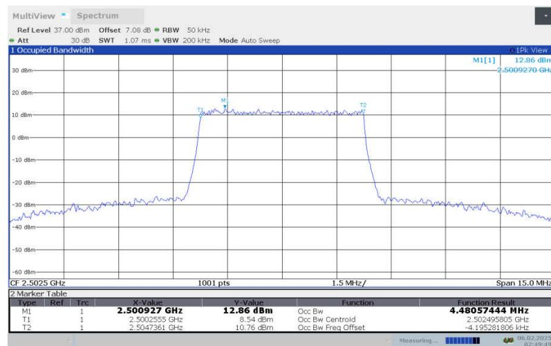
**LTE Band 7 , 5MHz Bandwidth,LOW,64QAM (99% OBW)**
