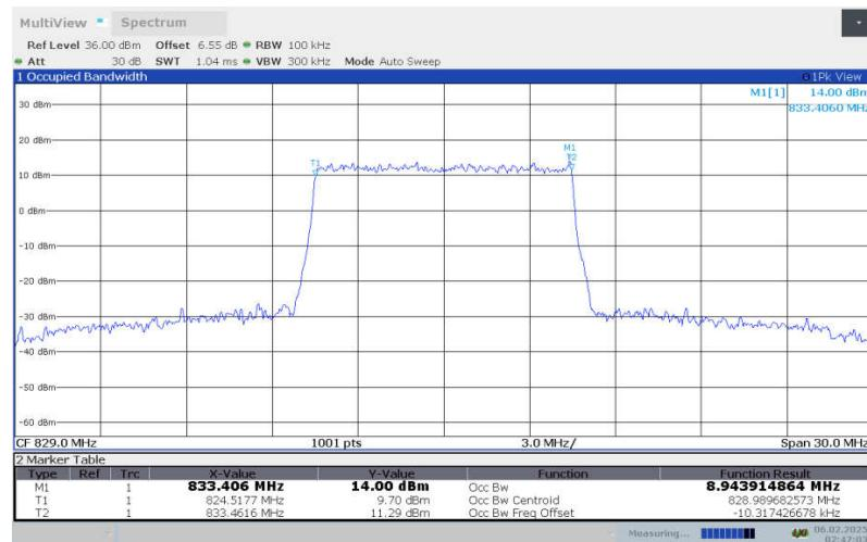
**LTE Band 5 , 10MHz Bandwidth,LOW,64QAM (99% OBW)**
