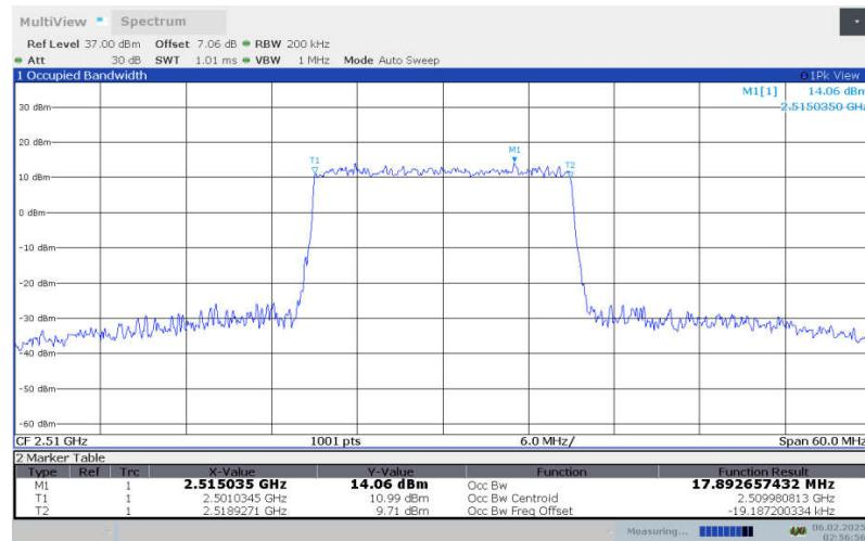
**LTE Band 7 , 20MHz Bandwidth,LOW,16QAM (99% OBW)**
