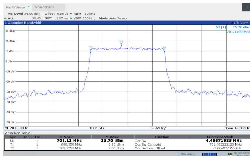
**LTE Band 12 , 5MHz Bandwidth,LOW,64QAM (99% OBW)**
