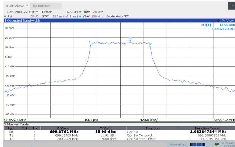
**LTE Band 12 , 1.4MHz Bandwidth,LOW,16QAM (99% OBW)**
