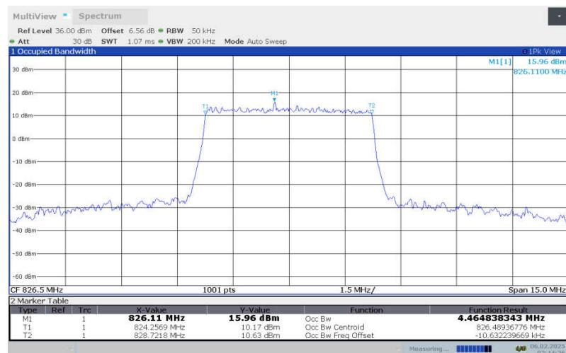
**LTE Band 5, 5MHz Bandwidth,LOW,64QAM (99% OBW)**
