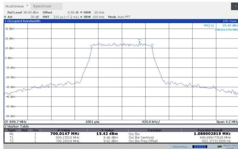
**LTE Band 12 , 1.4MHz Bandwidth,LOW,64QAM (99% OBW)**
