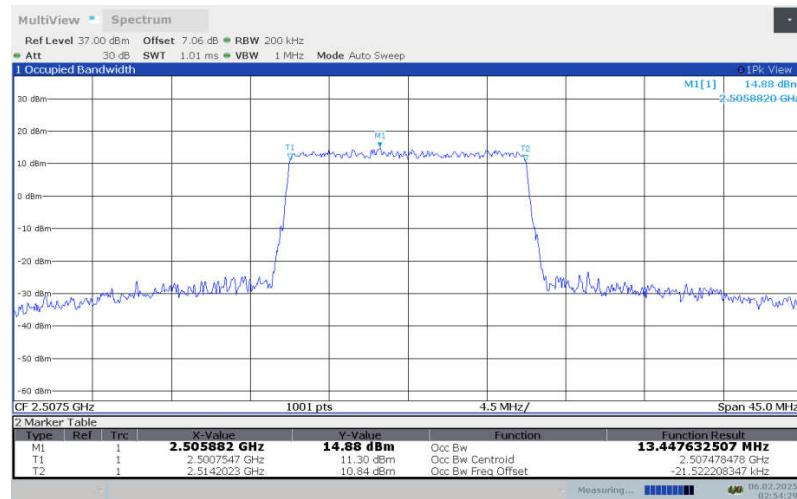
**LTE Band 7 , 15MHz Bandwidth,LOW,16QAM (99% OBW)**
