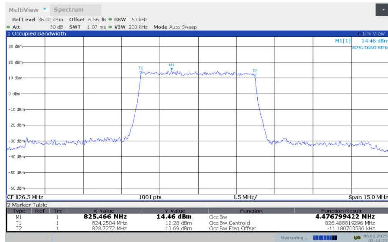
**LTE Band 5, 5MHz Bandwidth,LOW,16QAM (99% OBW)**
