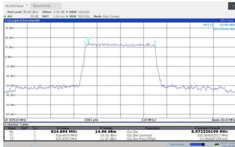
**LTE Band 5 , 10MHz Bandwidth,LOW,16QAM (99% OBW)**
