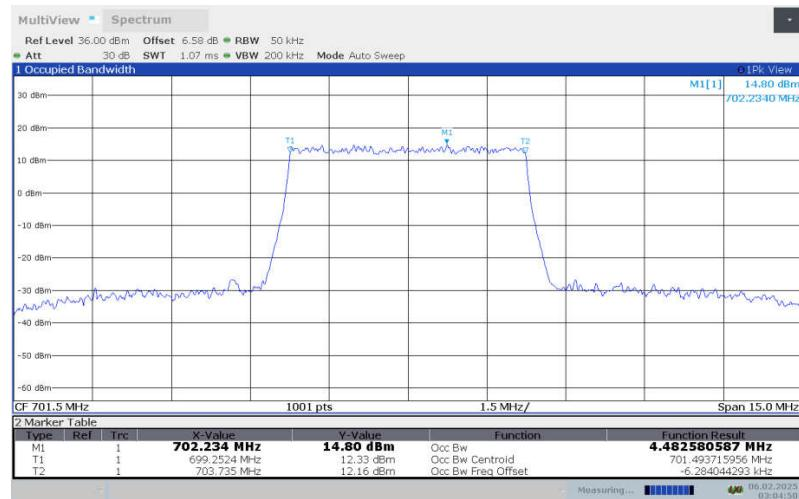
**LTE Band 12 , 5MHz Bandwidth,LOW,16QAM (99% OBW)**
