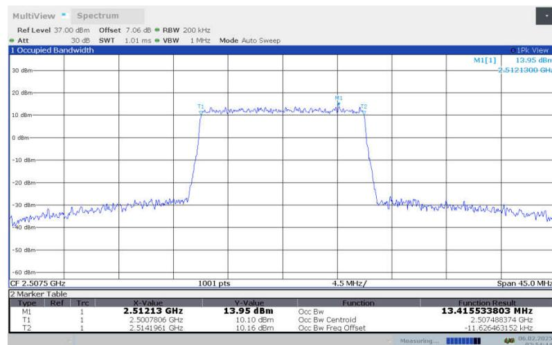
**LTE Band 7 , 15MHz Bandwidth,LOW,64QAM (99% OBW)**
