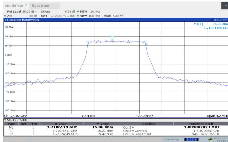
**LTE Band 4 , 1.4MHz Bandwidth,LOW,16QAM (99% OBW)**
