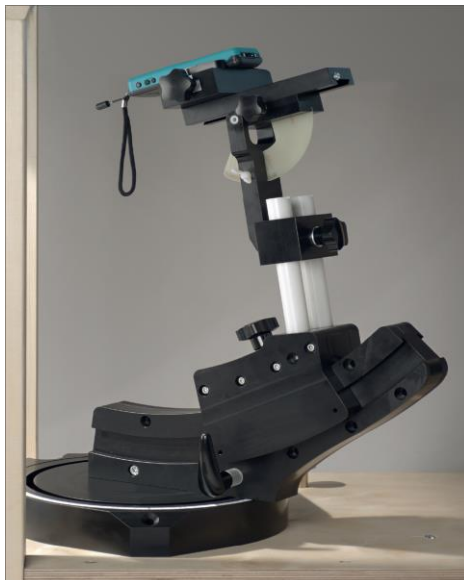
F-2. Device Holder for Transmitters
