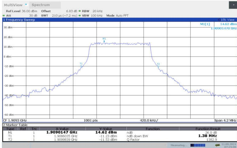
**LTE Band 2 , 1.4MHz Bandwidth,HIGH,16QAM (-26dBc BW)**
