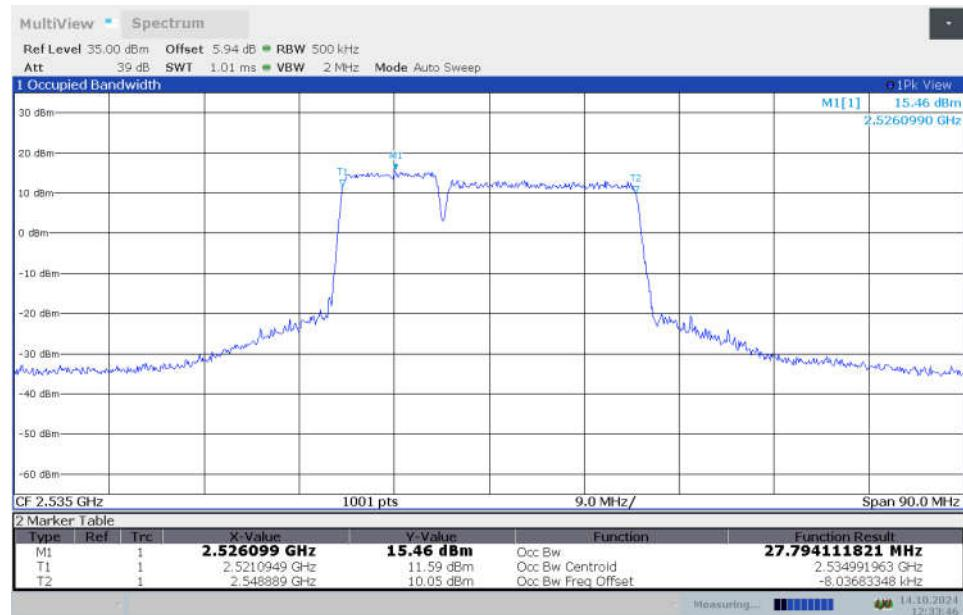
**LTE CA \_7C , 10MHz+20MHz Bandwidth,16QAM (99% BW)**
