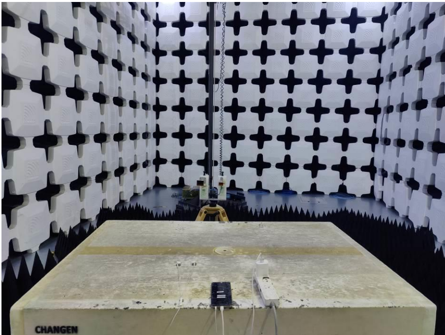
4. Radiated Emissions (Part 15B, Camera/LTE receiver, 26.5GHz-40GHz)
