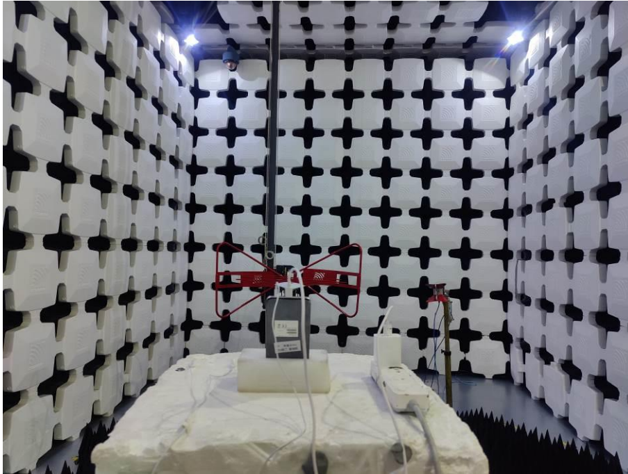
1. Radiated Emissions (Part 22/24/27, 30MHz-18GHz)
