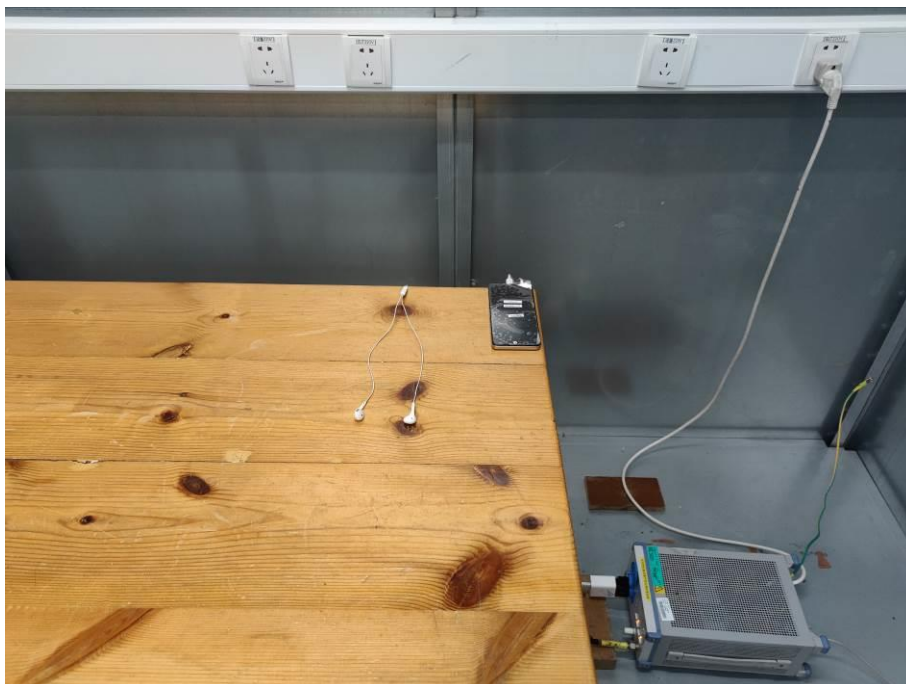
4. Conducted Emission (Part 15B, Camera/Video Player)
