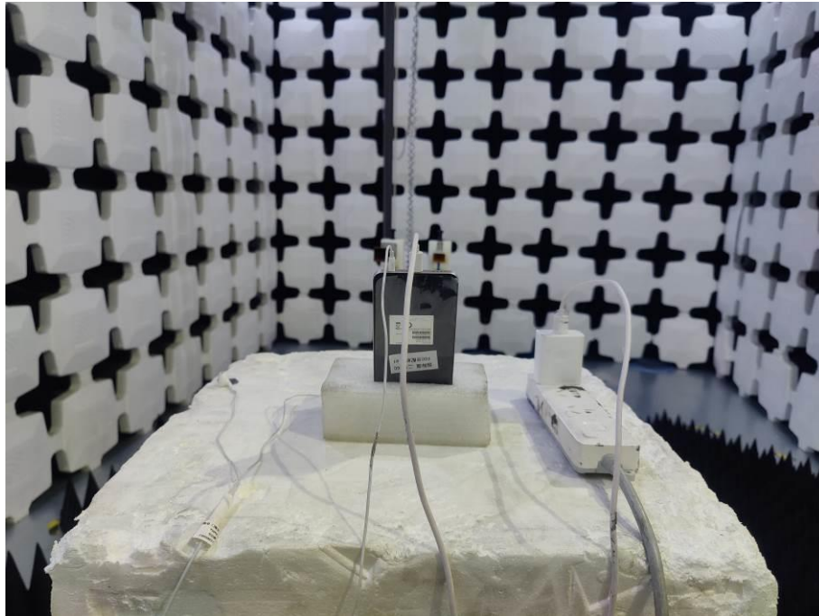
3. Radiated Emissions (Part 22/24/27, 26.5GHz-40GHz)
