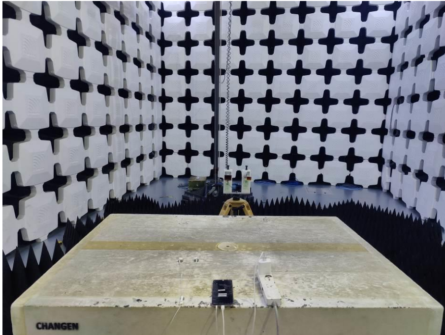
3. Radiated Emissions (Part 15B, Camera/LTE receiver, 18GHz-26.5GHz)
