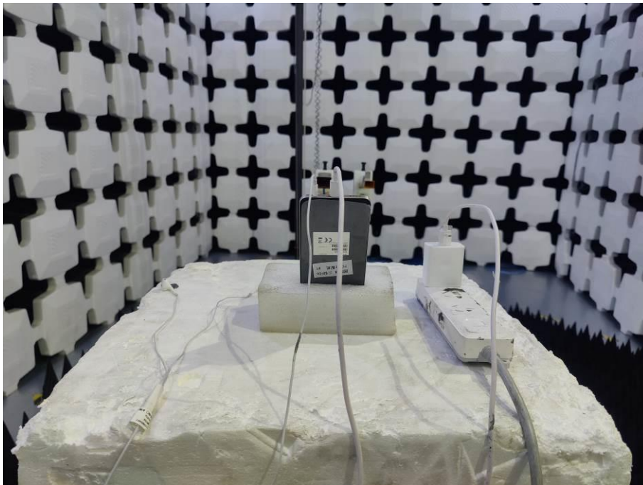
2. Radiated Emissions (Part 22/24/27, 18GHz-26.5GHz)
