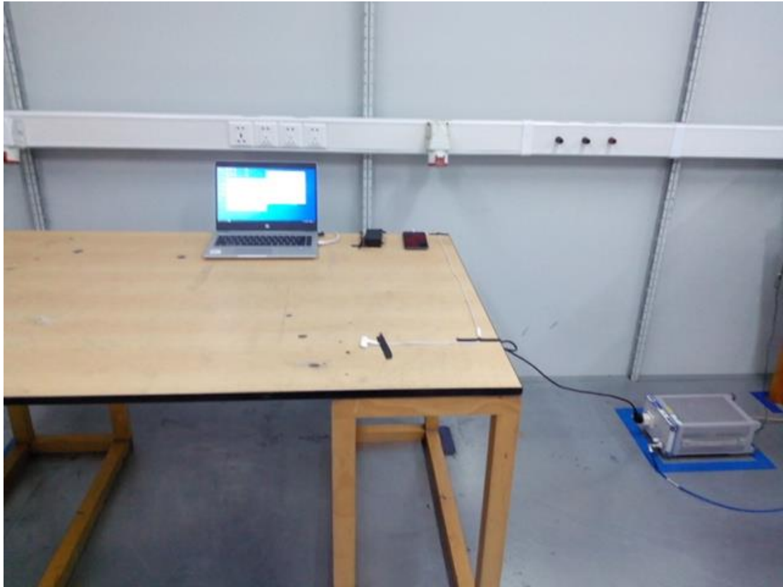
AC Conducted Emission Test Setup -Front
