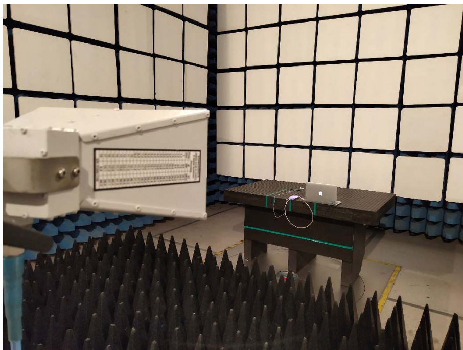
Above 1 GHz, The USB Test Mode
