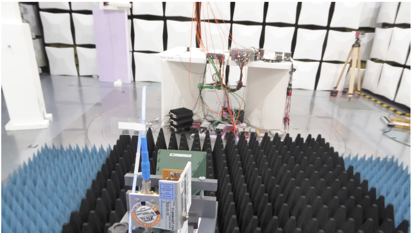
Test setup - Semi anechoic chamber with ground absorbers 18 GHz – 26.5 GHz
