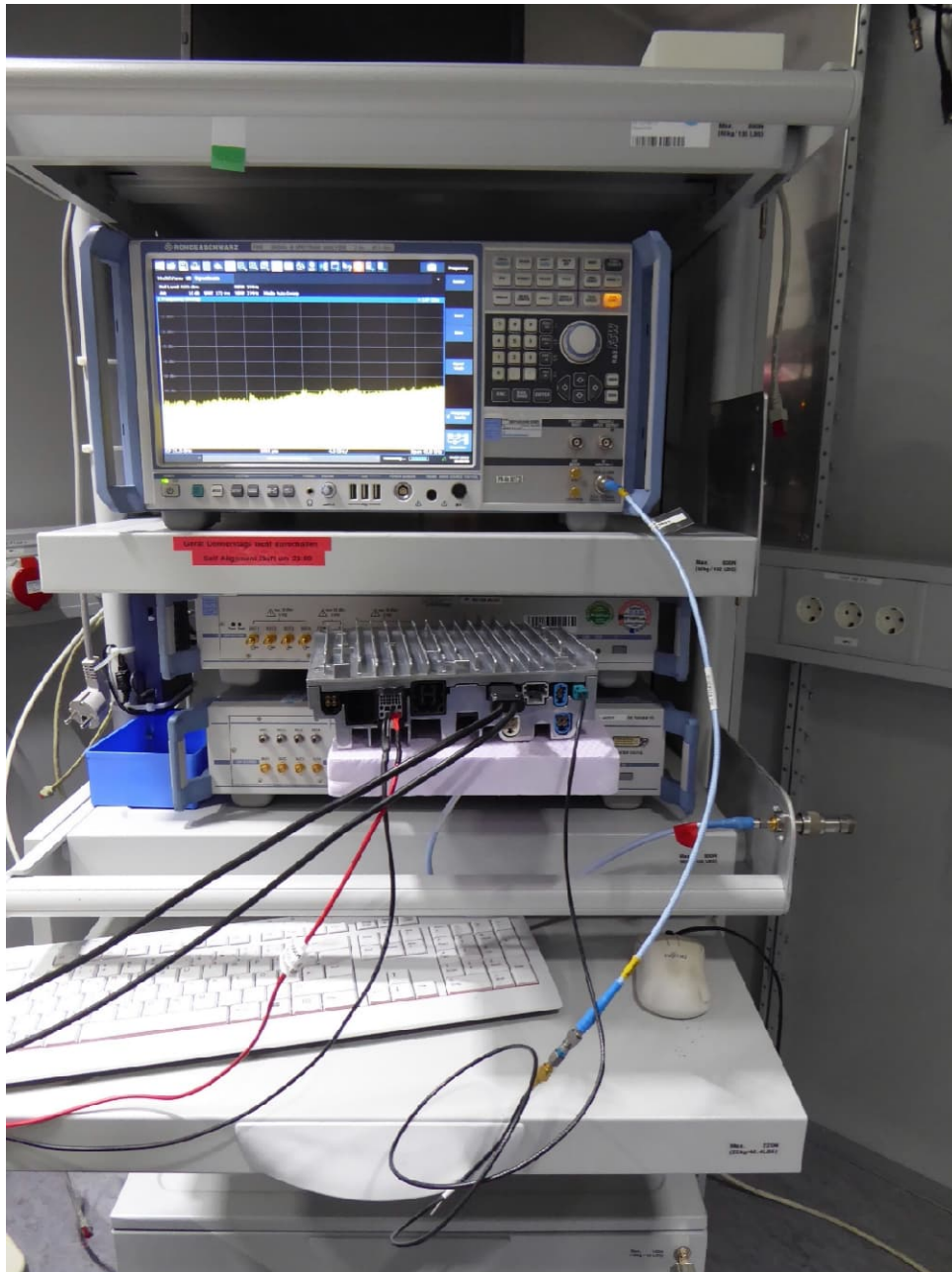
Test setup antenna port conducted – external antenna
