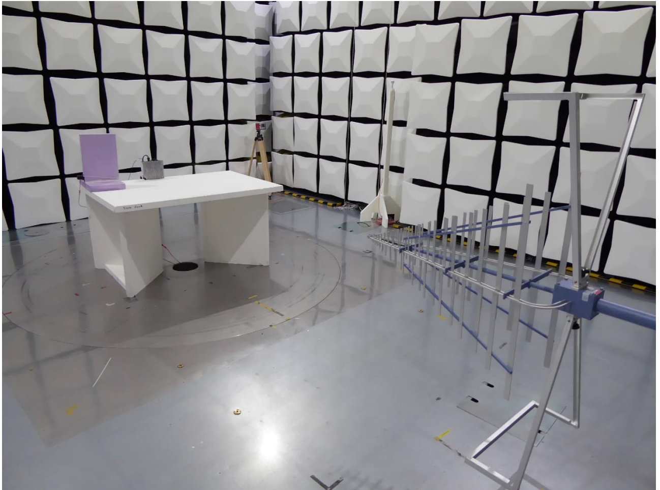
Test setup semi anechoic chamber (30 MHz – 1 GHz)
