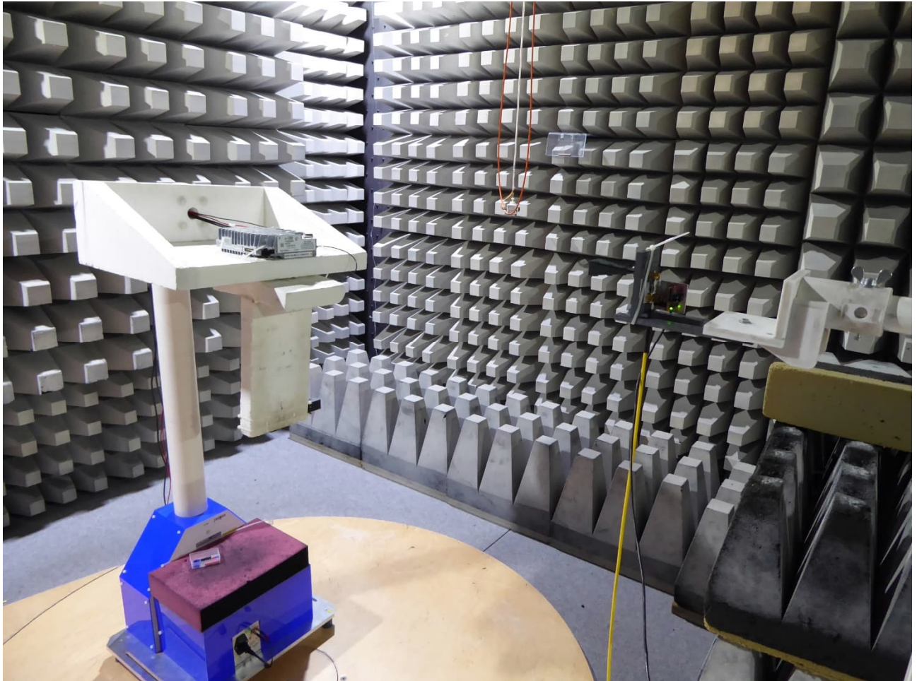
Test setup fully anechoic chamber (26.5 - 40 GHz)
