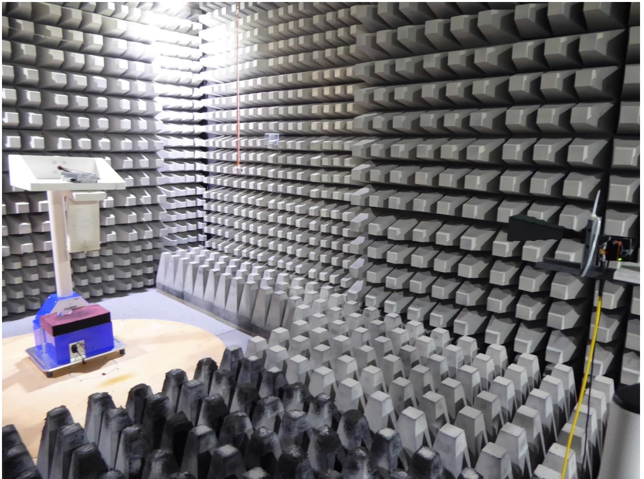
Test setup fully anechoic chamber (12 - 18 GHz)
