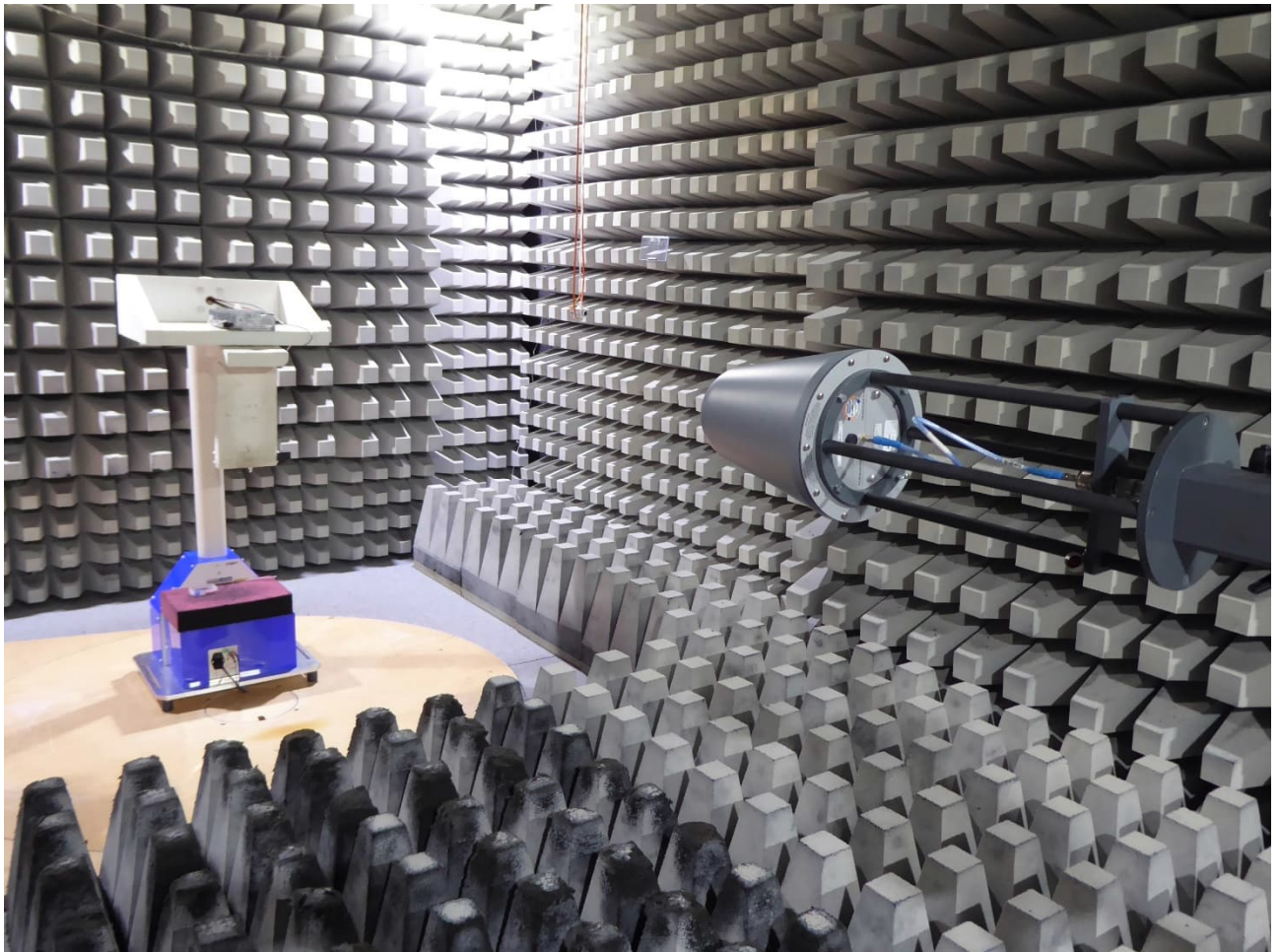
Test setup fully anechoic chamber (1 – 12 GHz)
