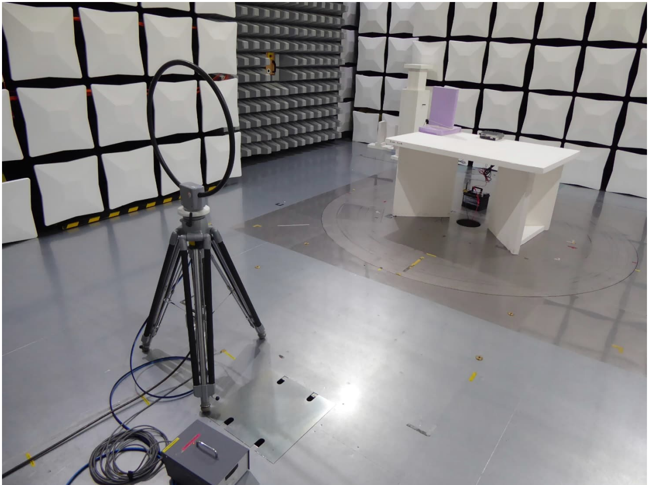
Test setup semi anechoic chamber (9 kHz – 30 MHz)
