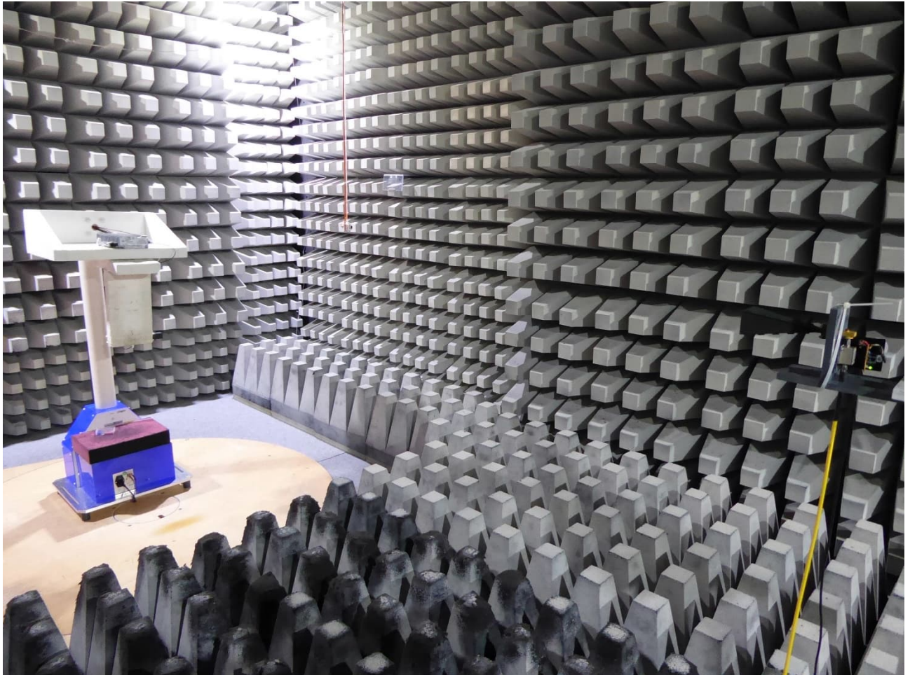
Test setup fully anechoic chamber (18 – 26.5 GHz)
