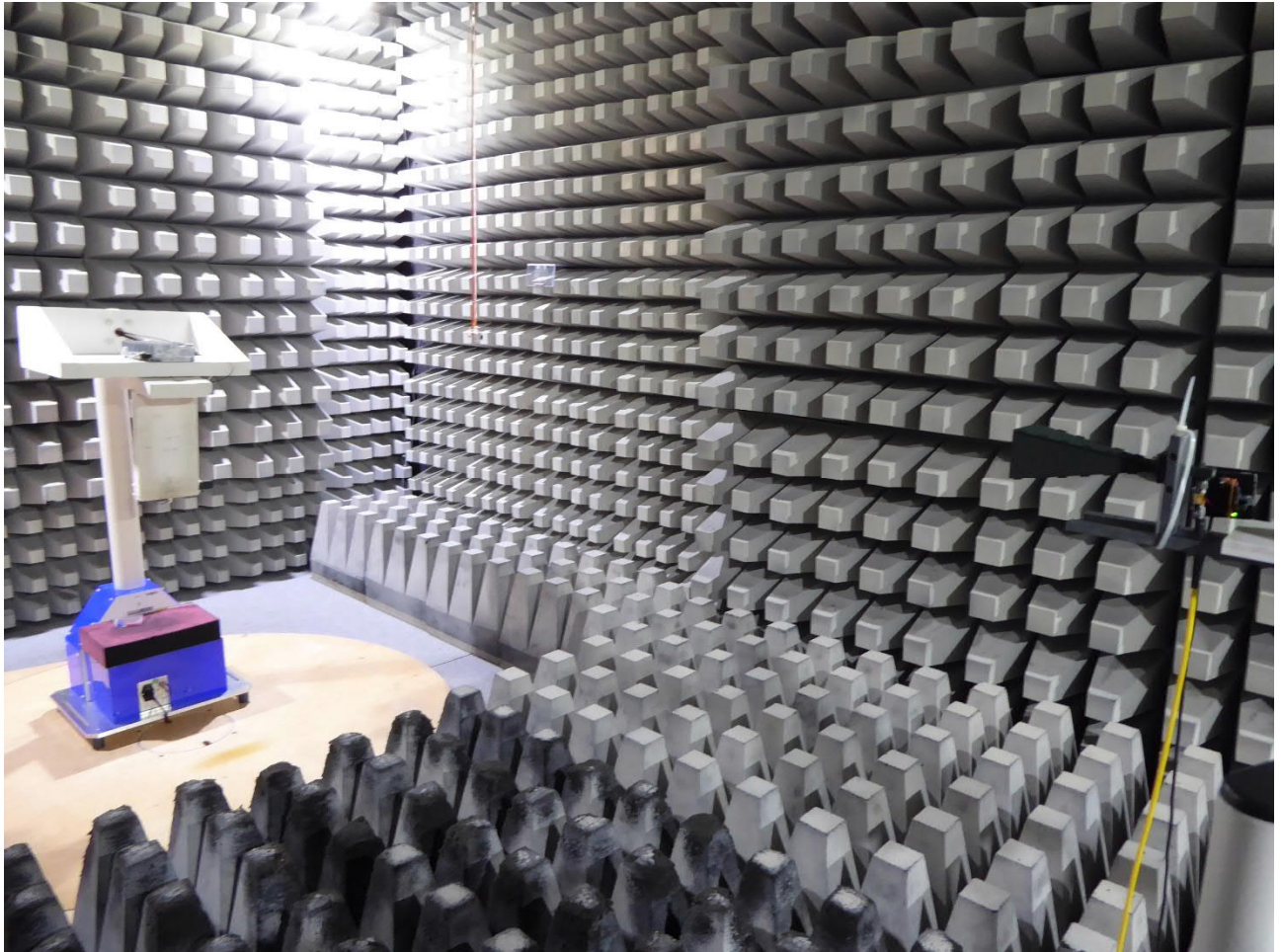
Test setup fully anechoic chamber (12 - 18 GHz)
