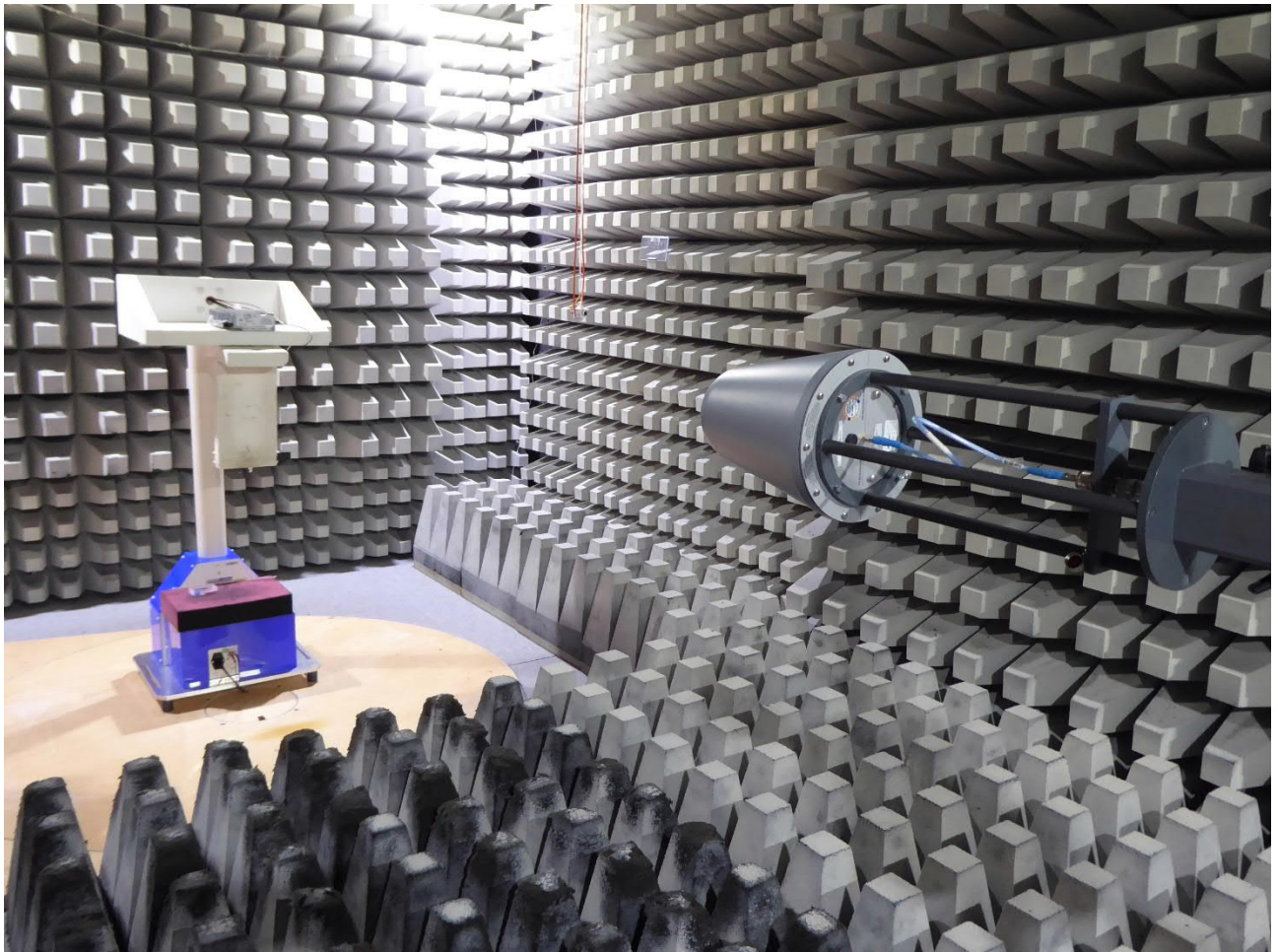
Test setup fully anechoic chamber (1 – 12 GHz)
