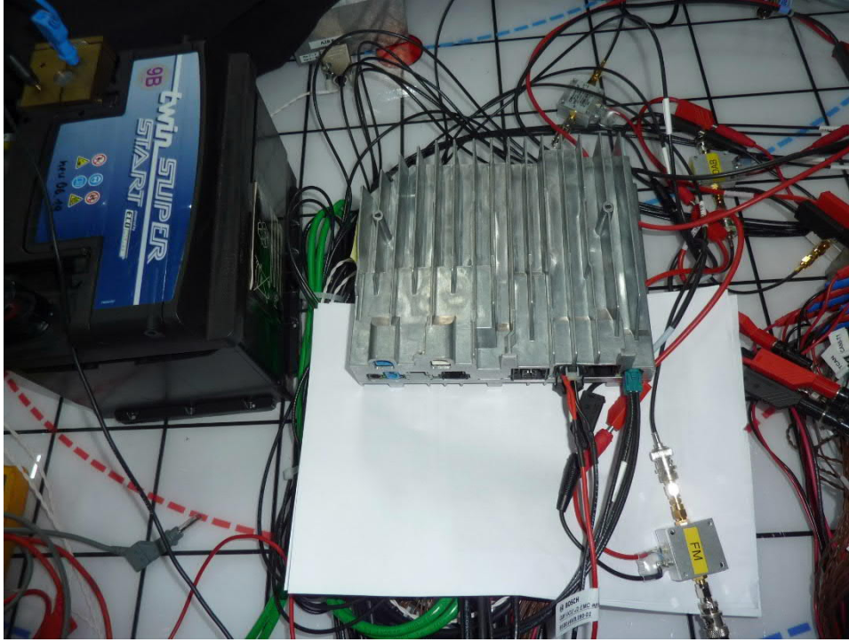
212286_27 Test setup conducted emission
