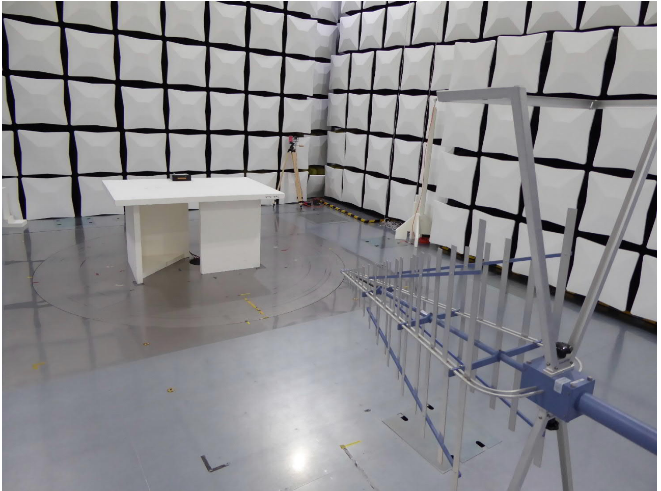
Test setup semi anechoic chamber
