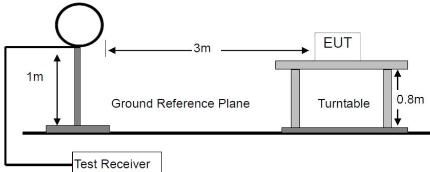
For Radiated Emission 30-1000MHz
