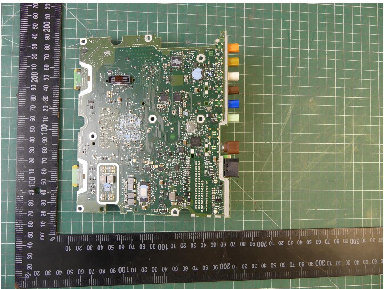
Bluetooth Antenna is integrated as printed circuit board antenna. It is Located as shown below:
