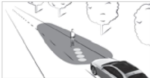
The spotlight function runs in the background and flashes the headlamps in four short bursts at persons detected within the lane markings. You will also be made aware of the position of the person by a projected symbol.
