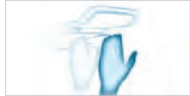
Hand movement to operate the roller sunblind and sliding sunroof
