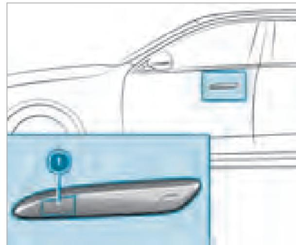
▶ **Lock and unlock the vehicle with the NFC function:** Hold the digital vehicle key against ❶ the door handle in the area of the NFC antenna.
