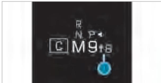
▶ When gearshift recommendation ① appears on the driver's display, shift to the recommended gear.
