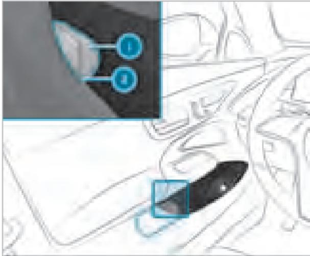
The safety vests are located in the safety vest compartments of the door compartment of all doors, under the armrests.
