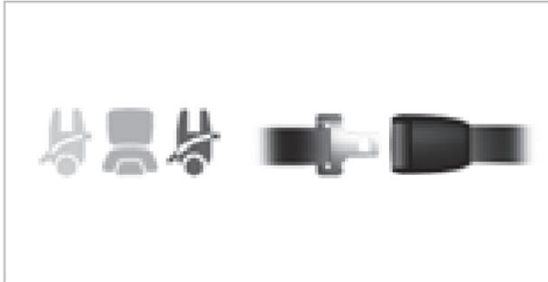
Depending on the vehicle equipment, you can determine the status of the rear seat belt by the colour of the seat symbol in the driver's display as follows:
