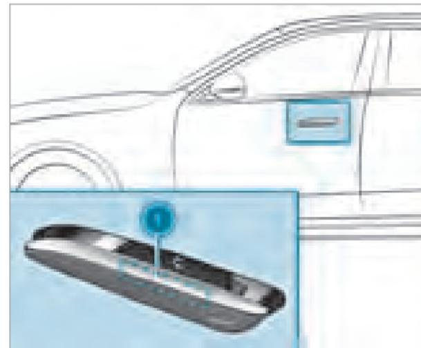
▶ **Unlocking the vehicle:** With the door handle extended, touch the inside surface **1** of the door handle.
