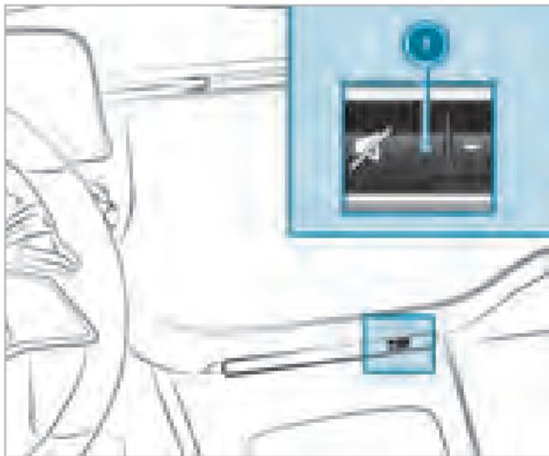
Indicator lamp ① flashes when the ATA system is primed.
