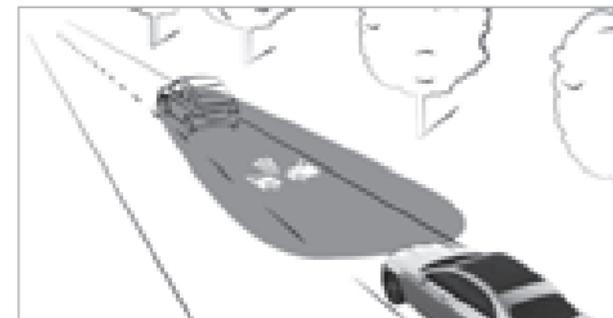
If you fall below the safe distance at speeds of at least 30 km/h, a collision warning symbol will be projected onto the road.
