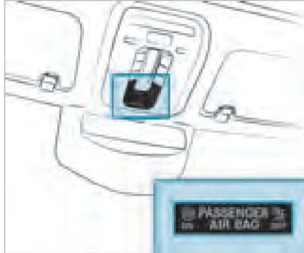
Vehicles without automatic front passenger airbag shutoff have a special sticker affixed to the side of the cockpit on the front passenger side (→ page 69).
