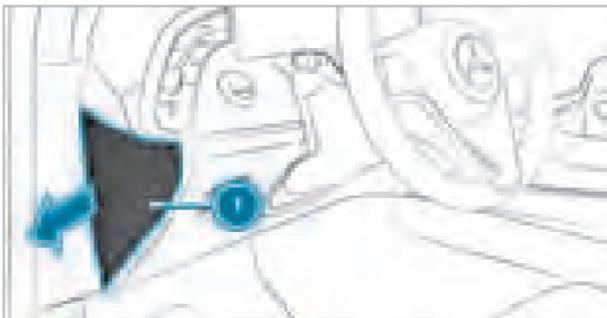
Fuse box ① is on the driver's side on the side of the cockpit under a cover.
