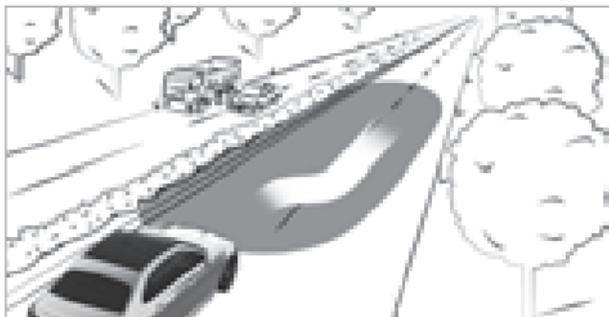
During assisted lane changes at speeds of at least 30 km/h, the course of the lane change as displayed will be brighter. This enables you to identify possible dangers in the new lane at an early stage.
