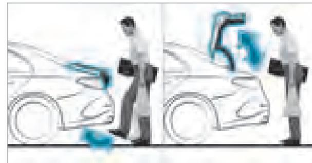
With HANDS-FREE ACCESS you can open, close or interrupt boot lid movement by performing a kicking movement under the rear bumper.
