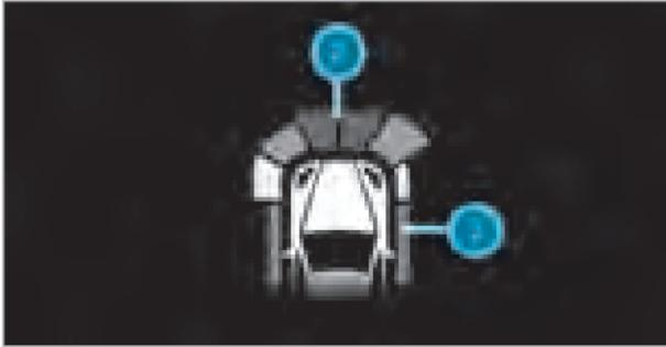
Optionally, obstacles detected by Parking Assist PARKTRONIC from a distance of approximately 1.0 m in front ② and 0.7 m on sides ③ can also be displayed in the head-up display.
