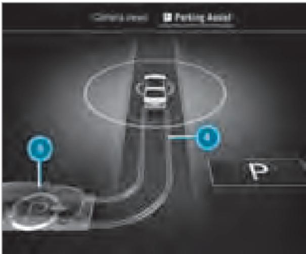
When the vehicle is stationary, indicated vehicle path ④ into currently selected parking space ⑤ also appears.
