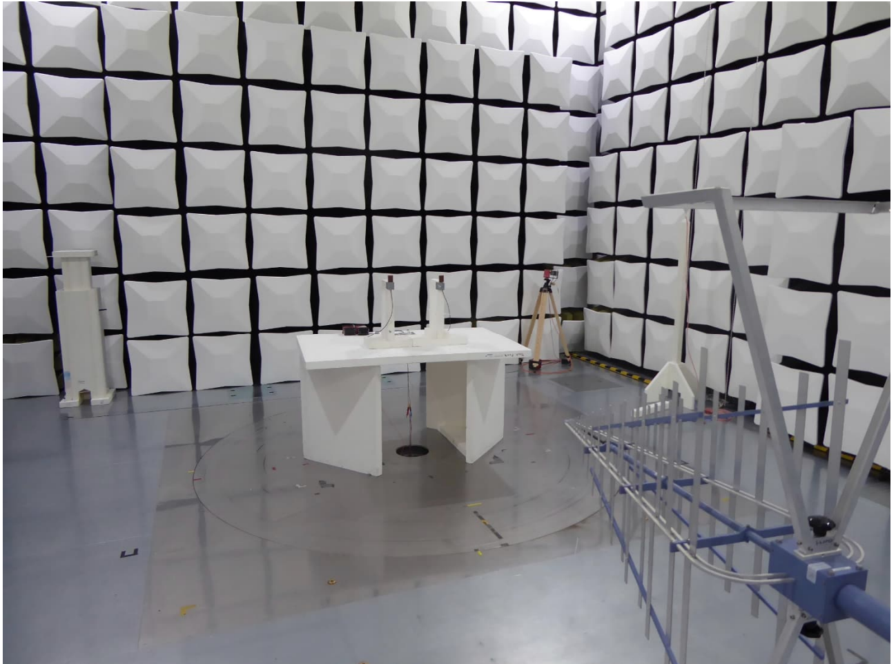
Test setup semi anechoic chamber (30 MHz – 1 GHz)
