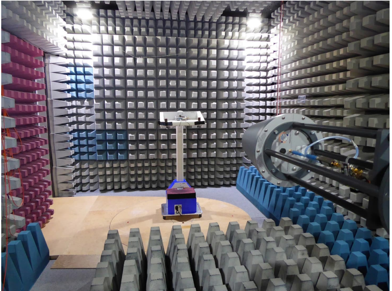
Test setup fully anechoic chamber (1 - 12 GHz)
