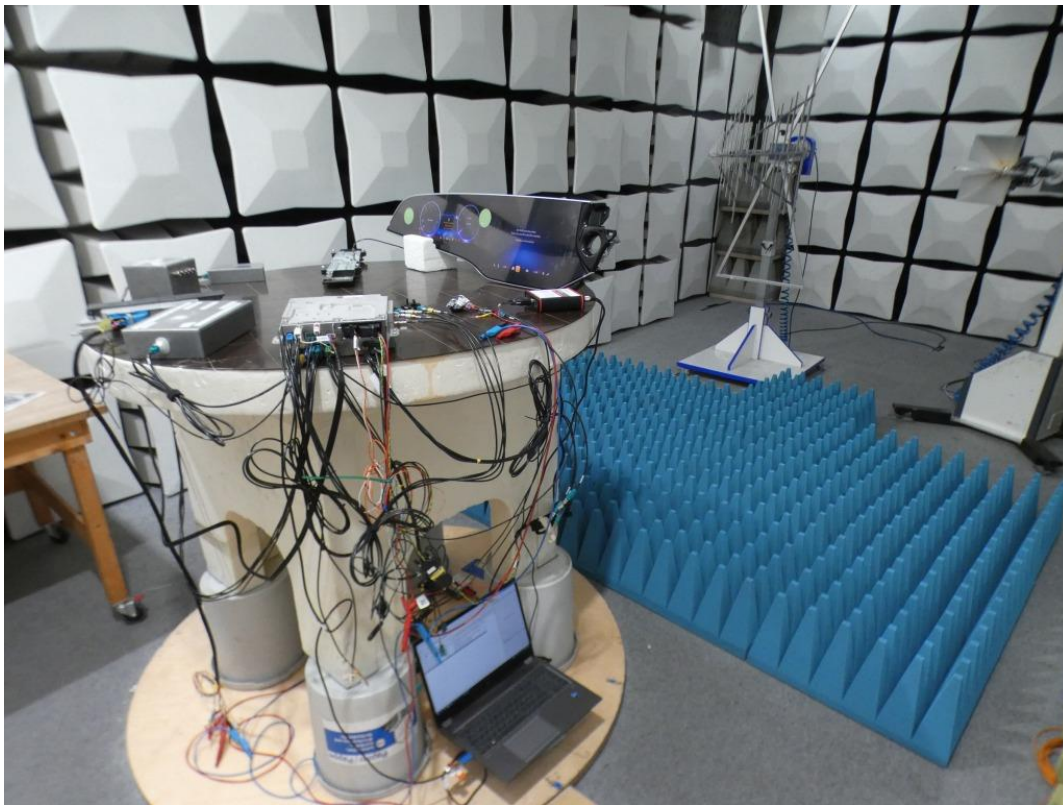
Photo 7: Test setup "Star 3.0" for radiated measurements (stand-alone, anechoic chamber 18 GHz – 26 GHz; unintentional radiator §15.109, ANSI C63.4)
