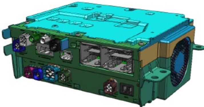
This product is built for two different vehicle architectures, thus being HW identical in all parts, one variant Star 3.0 uses CAN interface and lower GPU frequency, whereas Star3.5 uses vehicular ethernet with higher GPU frequency.
