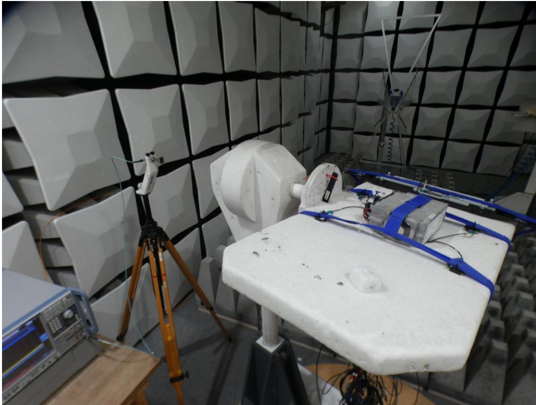
Photo 13: Test setup "Star 3.5 / Star 3.0" for radiated measurements, detailed view (above 1 GHz; Fully anechoic chamber, FCC Part 15.407; ANSI C63.10)
