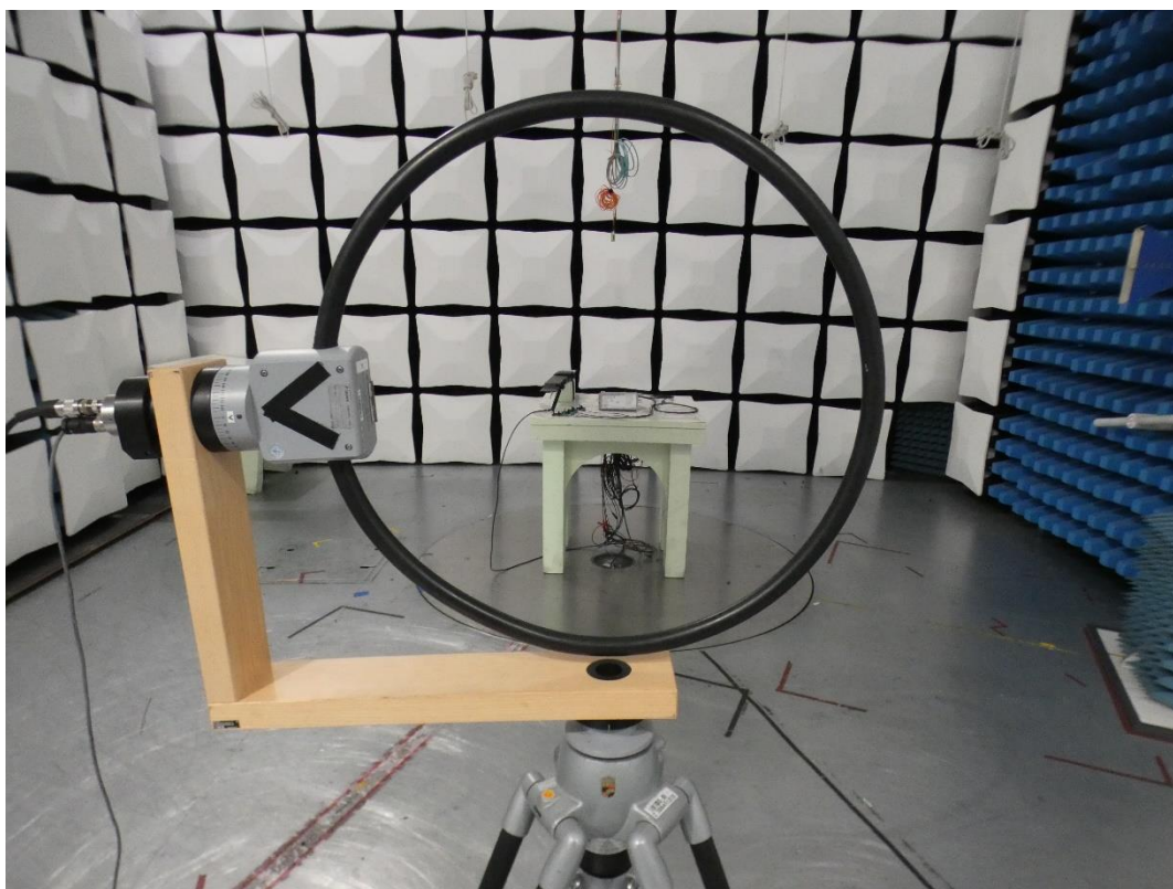
Photo 9: Test setup "Star 3.5 / Star 3.0" for radiated measurements (semi-anechoic chamber 9 kHz – 30 MHz; FCC Part 15.247 and 15.407, ANSI C63.10)
