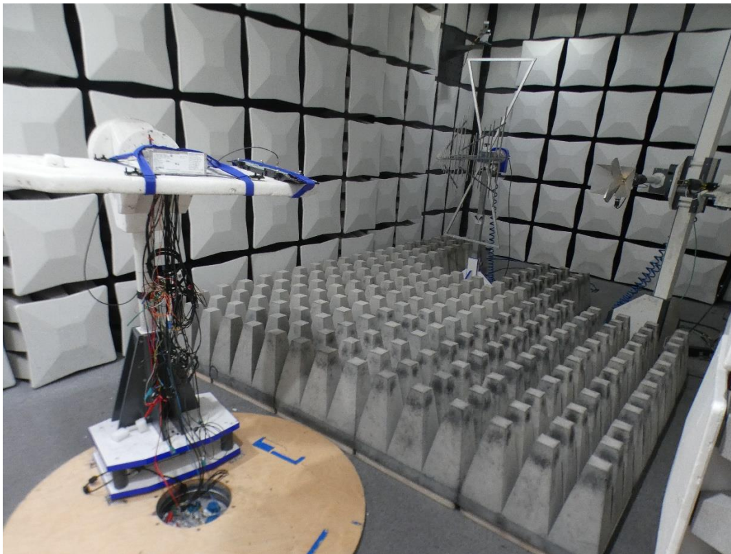
Photo 11: Test setup "Star 3.5 / Star 3.0" for radiated measurements (above 1 GHz; Fully anechoic chamber, FCC Part 15.247 and 15.407; ANSI C63.10)
