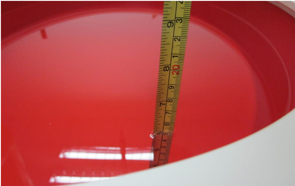
Figure 4.4: Liquid depth in the Flat Phantom
