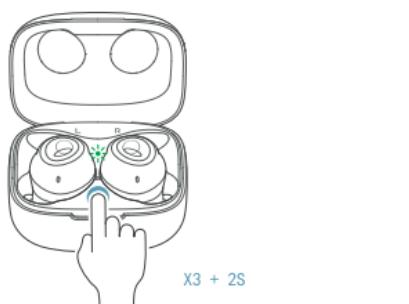
Place the Earbuds into the charging case and keep it open. press and hold the button in the case for 2 seconds until the LED indicator in the charging case flash green.
