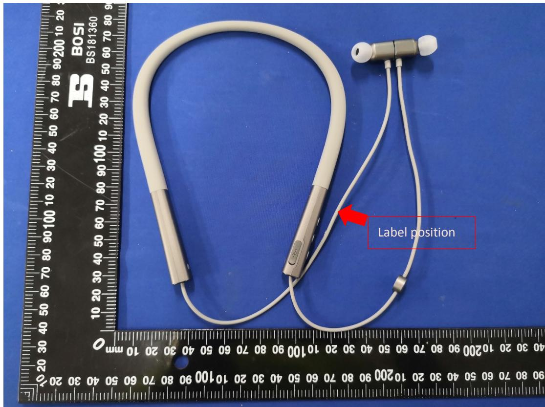
The FCC label is attached to the left earphone cable (the wire without the microphone), then the label is folded in half.
