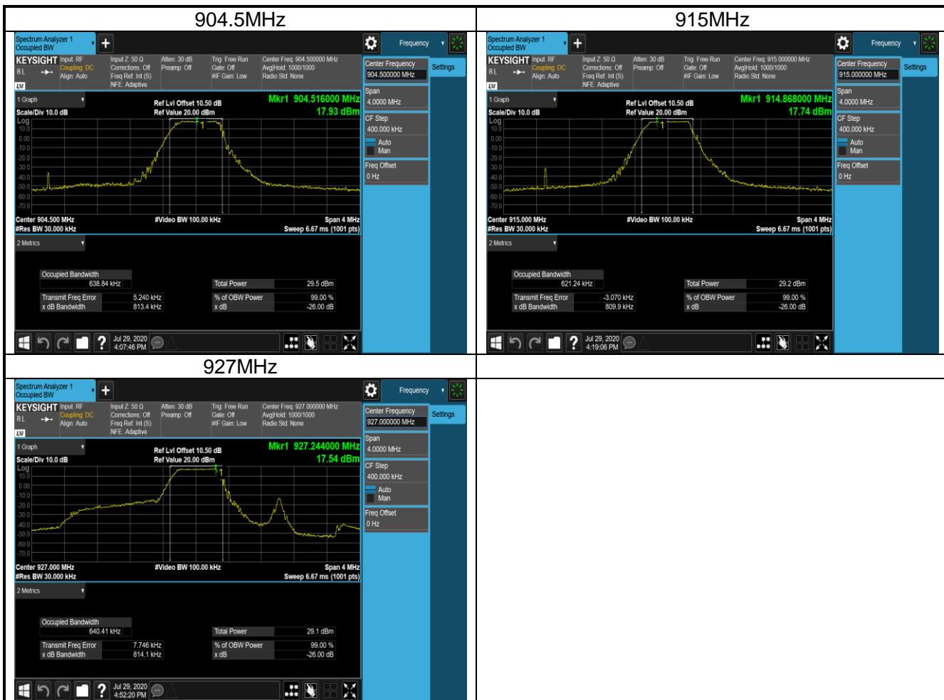
**TEST REPORT****Transmitter Spurious Emission****Test Result and Data**
