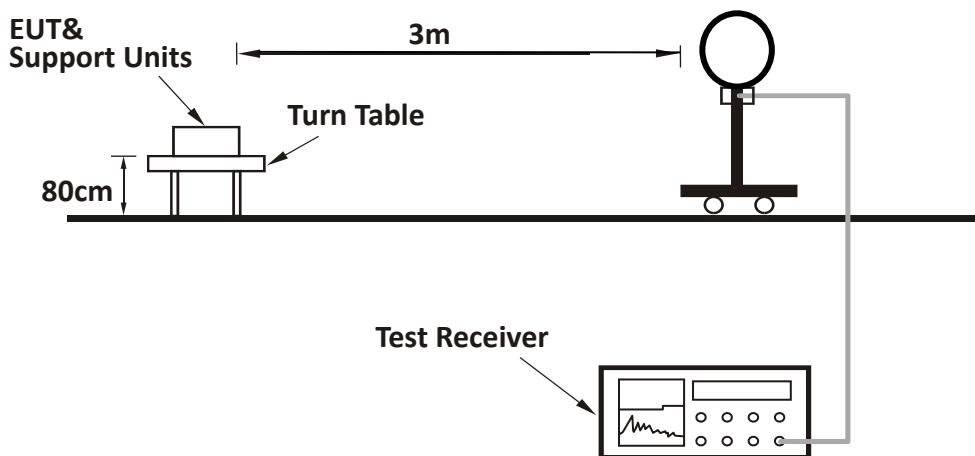
**For Radiated emission 30MHz to 1GHz:**
