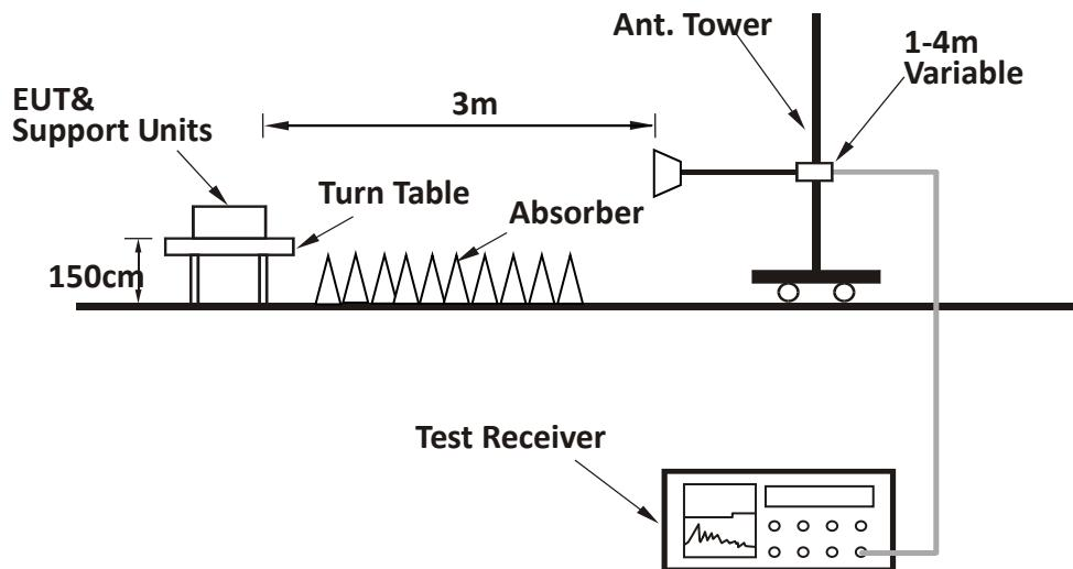
**TEST REPORT****7.4 Test Results of Radiated Emissions**
