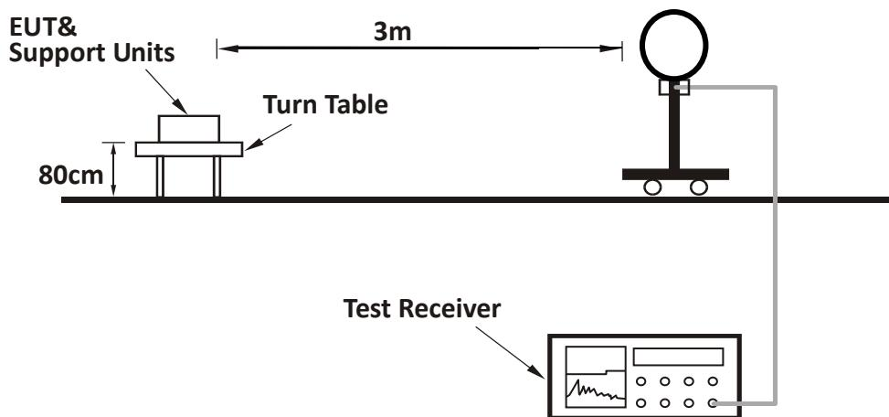
For Radiated emission 30MHz to 1GHz:
