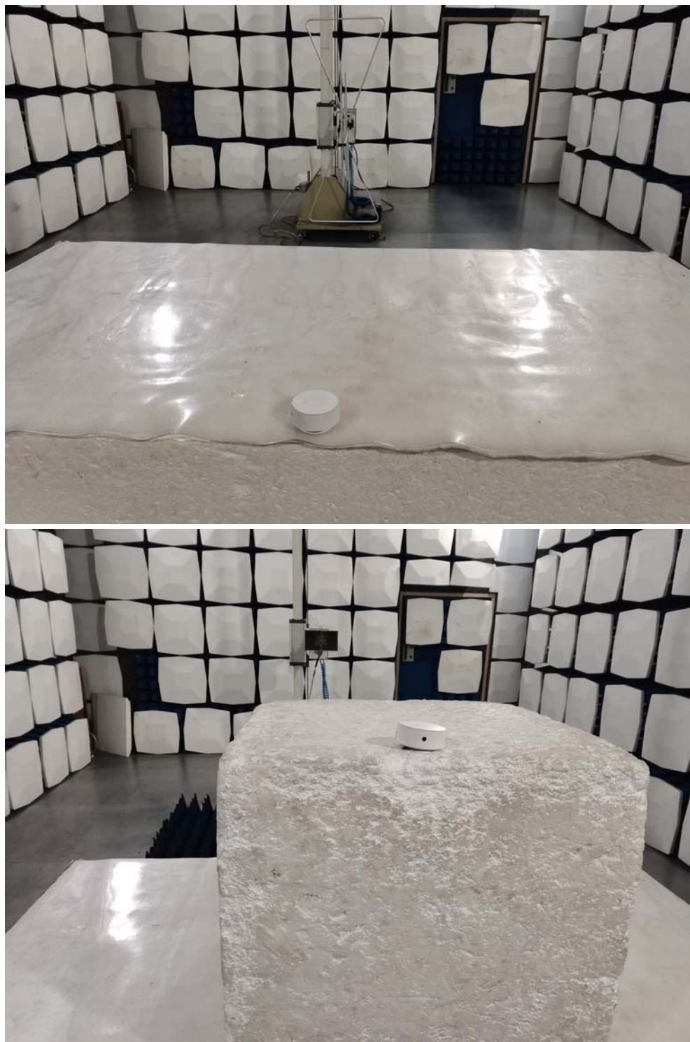
Radiated emission test view
