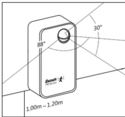
It is recommended that the installation height be 1~1.2m, less than 1m or greater than 1.2m, the detection range becomes smaller, blind areas appear, and some areas cannot be detected. When installing, please pay attention to the lens to be aligned with the area to be detected. When placing or pasting, the sensor should be as close as possible to the edge of the desktop or the edge of the cabinet.
