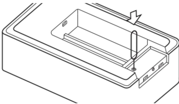
The device that has been successfully paired, the long stamp pairing button is 8s, and the device releases the current pairing relationship and re-enters the pairing state.
