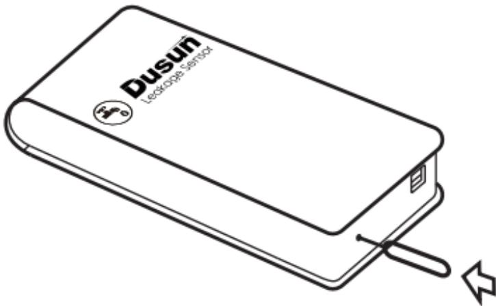
The device that has been successfully paired, the long stamp is paired with the hole for 8s, and the device releases the current pairing relationship and re-enters the pairing state.
