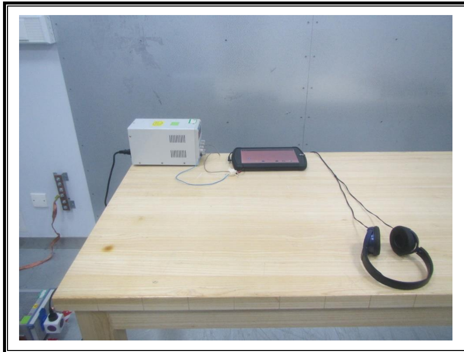
POWERLINE CONDUCTED EMISSIONS MEASUREMENT SETUP
