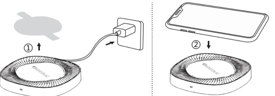
1. Remove the film on the charging pad and connect the power with QC adapter.
