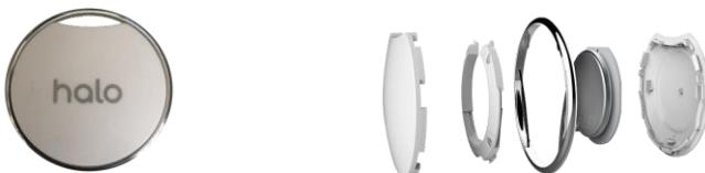
Turn on the Halo Beacon by pressing on the halo logo and holding for 3 seconds until the blue LED turns on - then release. To turn off, hold down again for 3 seconds - and confirm that - after releasing - the blue 'power' LED blinks 5 times.
