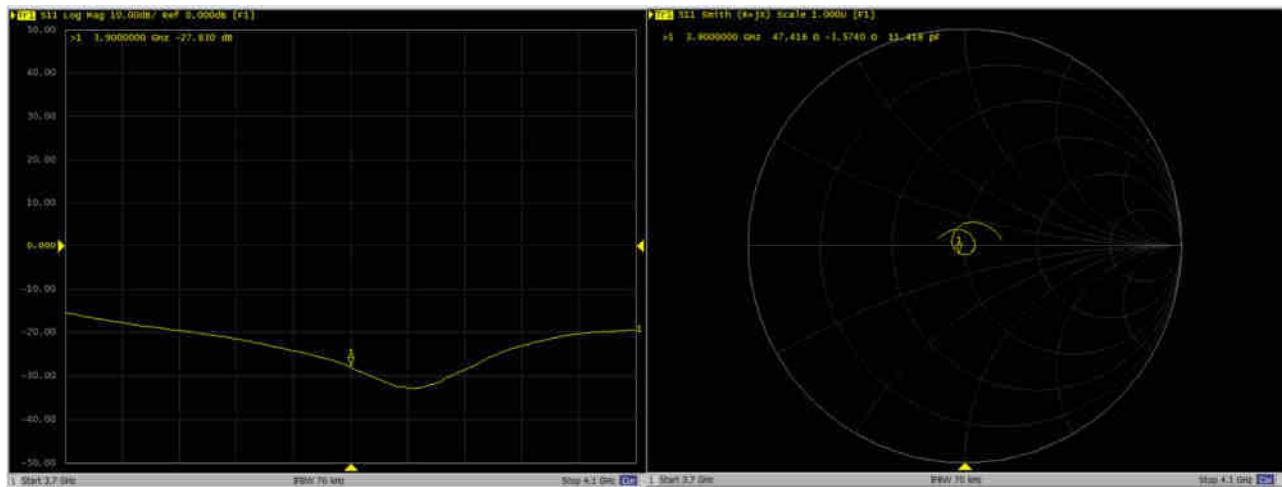
**Dipole Verification Data > D3900V2, serial no. 1048****4100MHz – Head----2025.3.7**
