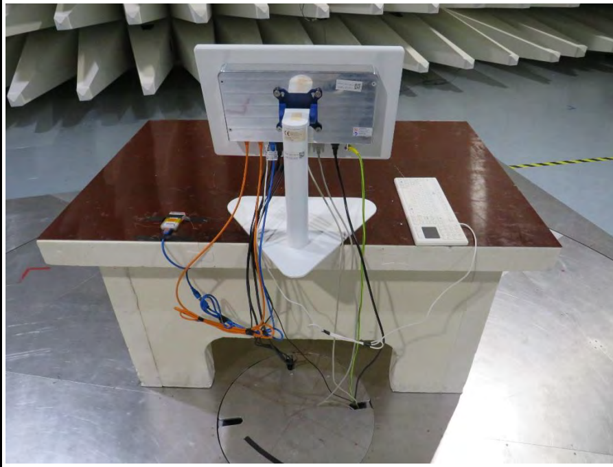
OR-PC® 21 Radiated Emission Test Setup 30 - 1000 MHz
