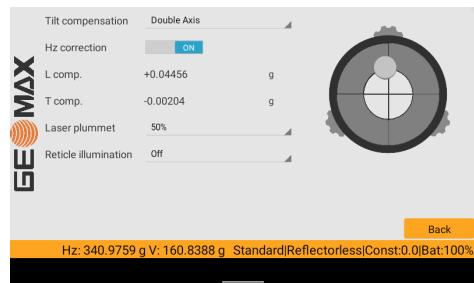
3. When the electronic level is centered and both axes are within the tolerance limit, the instrument has been levelled up.
