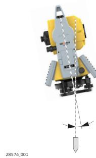
Angle between plumb line and standing axis.
