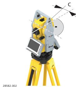
The line-of-sight error ( $c$ ) is the deviation from the perpendicular between the tilting axis and line of sight. This could be eliminated by measuring in both faces.
