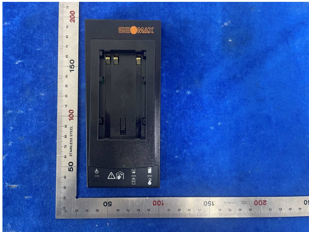
Picture 51: View of the battery charge base
