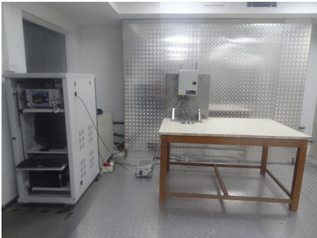
Photo 12: Conducted emission test on AC Line test setup
