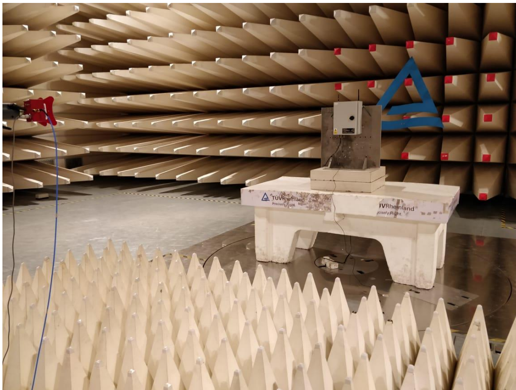
Photo 11: 18GHz to 26.5GHz-Horizontal polarization
