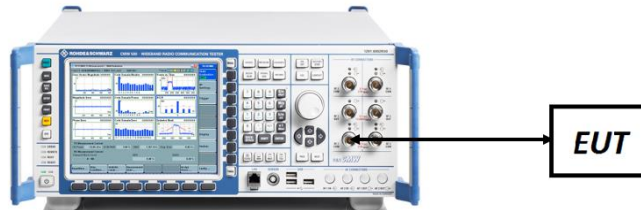
Figure 7-1. Conducted Power Measurement Setup
