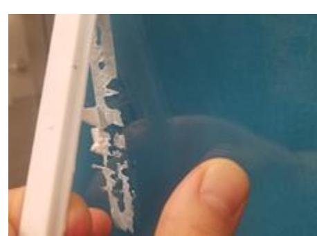
When you have loosened the adhesive enough you can carefully remove it by hand.
