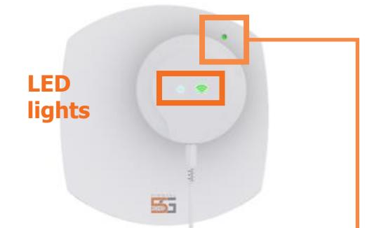
Plug the Echo 5G IDU into your wall outlet. Blue and green LED lights on the IDU will appear and blink before going solid. If the green light blinks for more than 30 seconds, consult the Troubleshooting Help on the back of this page.
