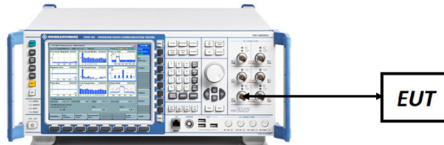
Figure 7-1. Conducted Power Measurement Setup
