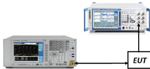
Figure 6-1. Test Instrument & Measurement Setup
