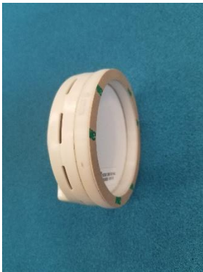
Assembled IDU, spacer ring, and Velcro-to-window adhesive
