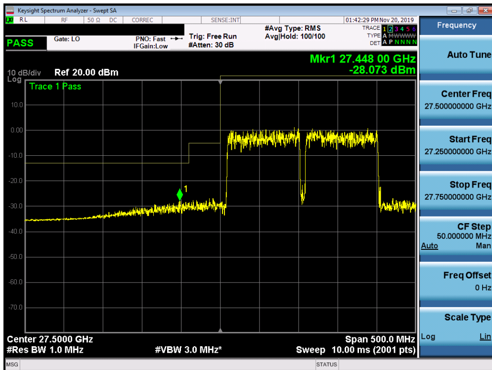
Plot 6-10. HBF Vertical Antenna Lower Band Edge Plot with 2 Carriers.
