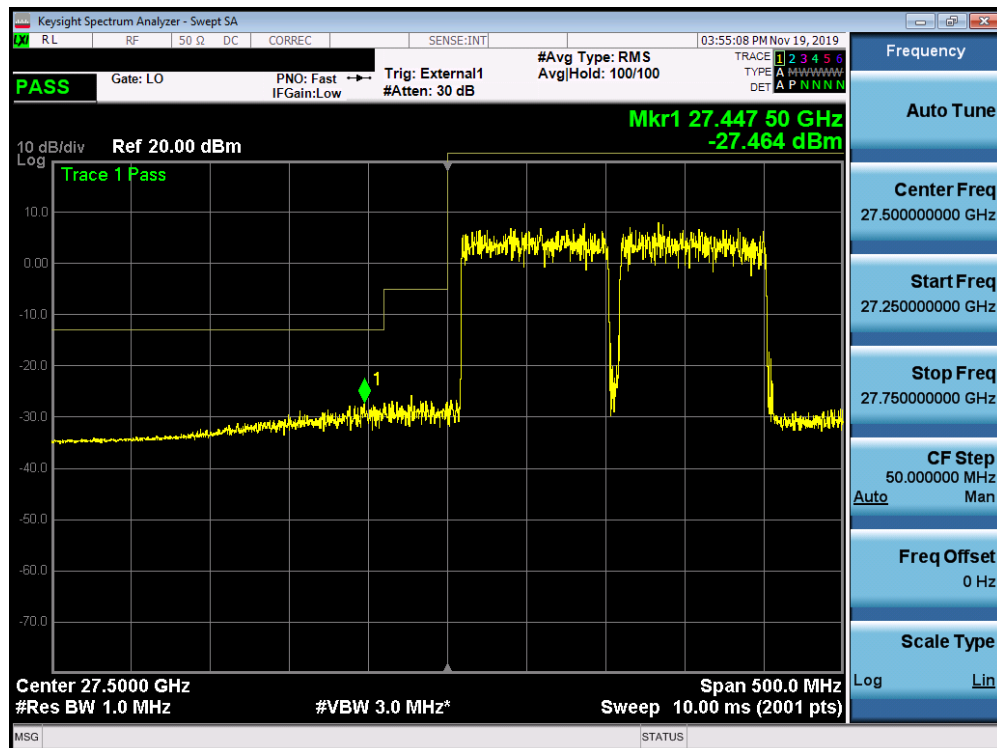
Plot 6-14. Patch Vertical Antenna Lower Band Edge Plot with 2 Carriers.
