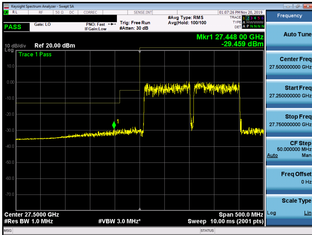
Plot 6-9. HBF Horizontal Antenna Lower Band Edge Plot with 2 Carriers.
