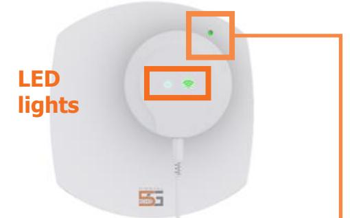
Plug the Echo 5G IDU into your wall outlet. Blue and green LED lights on the IDU will appear and blink before going solid. If the green light blinks for more than 30 seconds, consult the Troubleshooting Help on the back of this page.
