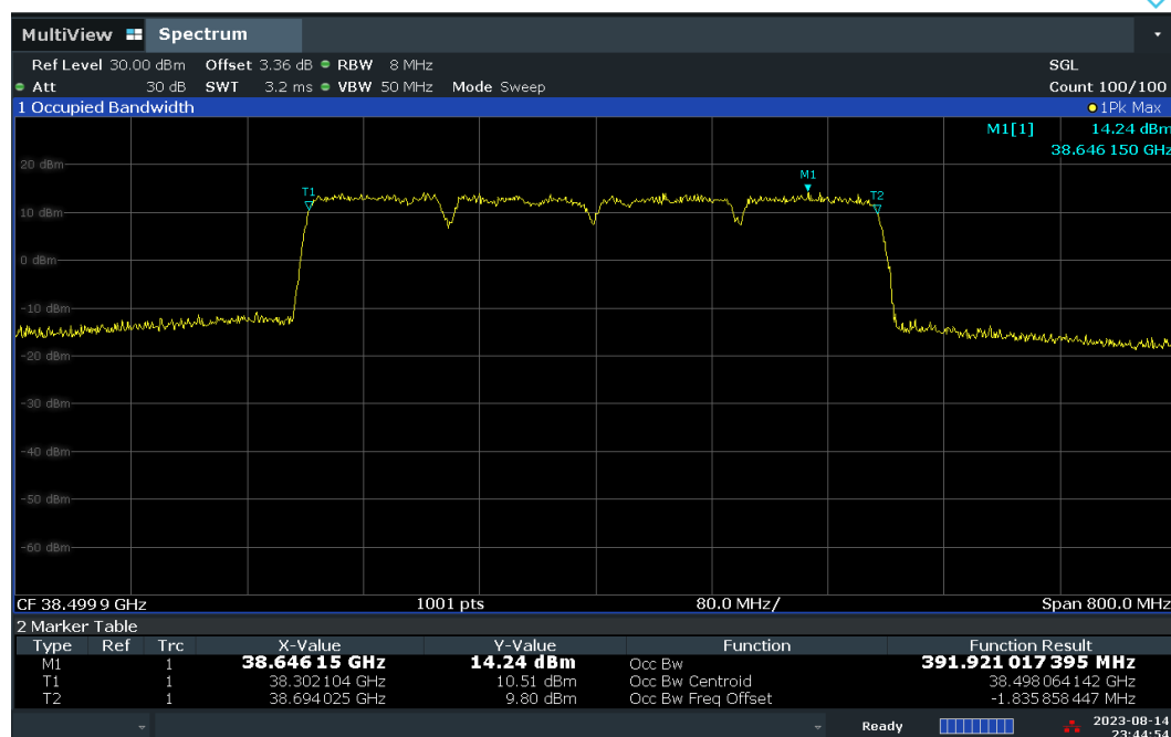
Plot 7-24. Occupied Bandwidth Plot – DFT-s – V-DL Polarization (100MHz-4CC – 16QAM – Mid Channel)
