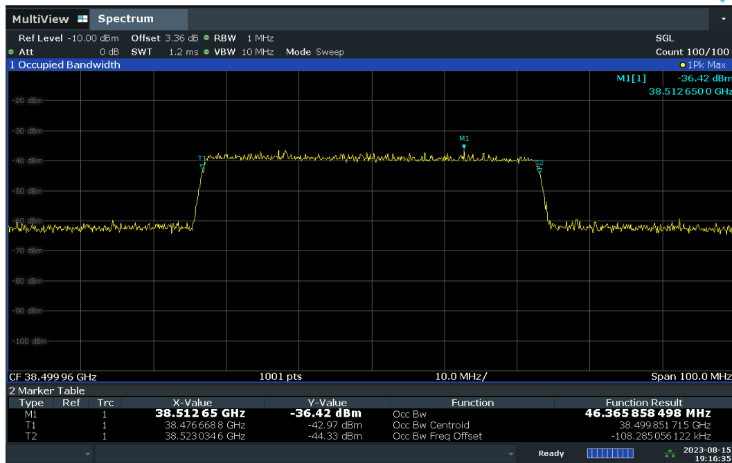
Plot 7-5. Occupied Bandwidth Input at 0.5dB below AGC Threshold – DFT-s – H-DL Polarization.
