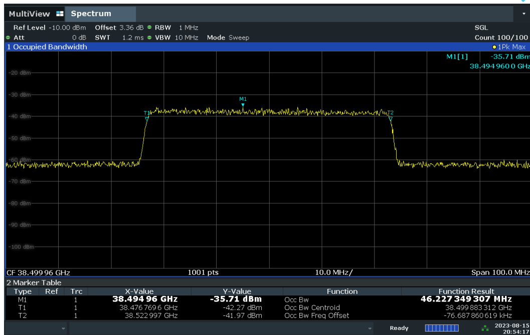
Plot 7-9. Occupied Bandwidth Input at 0.5dB below AGC Threshold – CP – V-DL Polarization.
