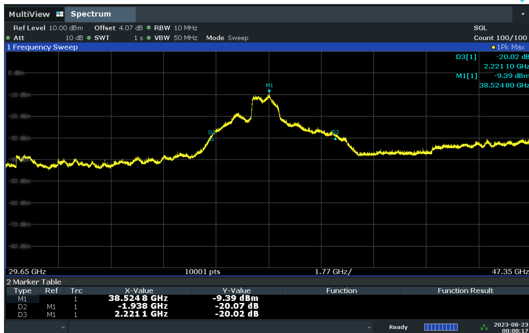
Plot 7-18. Out-Of-Band Rejection – H-DL Polarization
