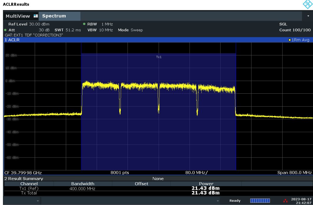
Plot 7-105. Conducted Power Plot – CP – V-DL Polarization (100MHz-4CC – 16QAM – High Ch. – Full RB)
