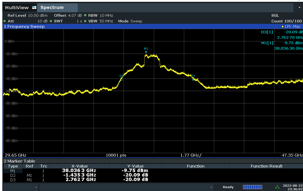
Plot 7-17. Out-Of-Band Rejection – V-DL Polarization
