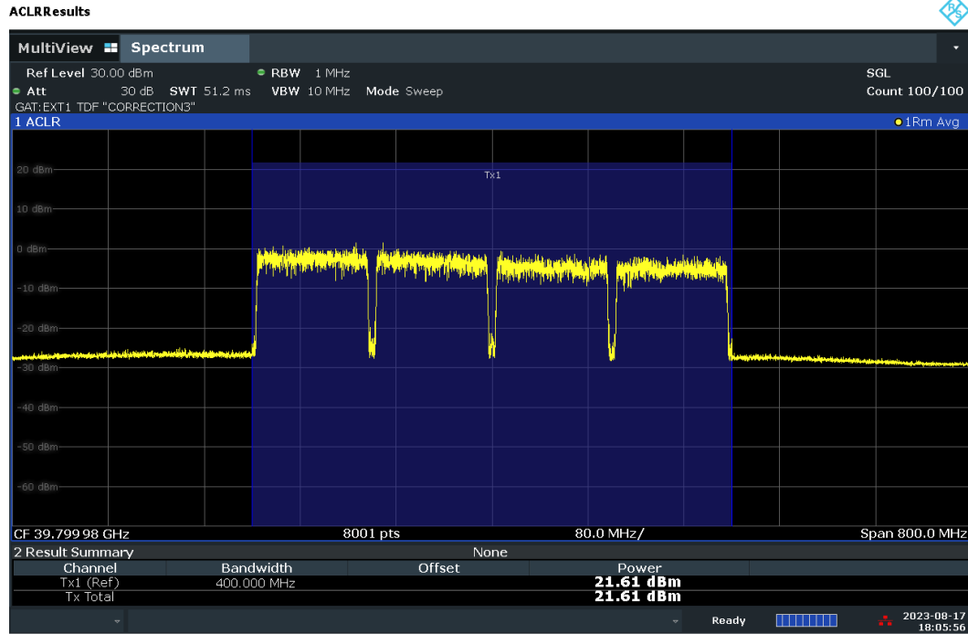
Plot 7-82. Conducted Power Plot – DFT-S – H-DL Polarization (100MHz-4CC – QPSK – High Ch. – Full RB)
