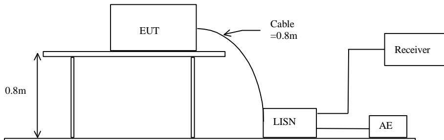
Remarks: The antenna of the EUT was terminated with 50 ohm resistive load
