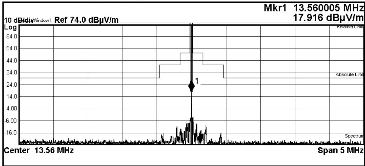
Total Power -27.85 dB $\mu$ V/m / 0.01 MHz Spectrum Peak Ref 84.00 dB $\mu$ V/m
