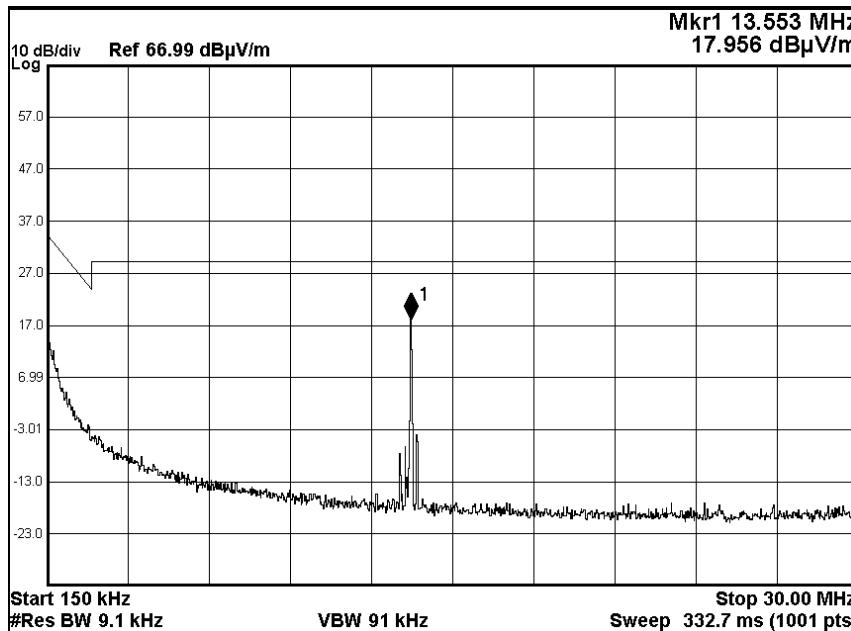
The peak value shown on the graph was 13.56MHz which the result was measured and calculated at page 7-8, others missions detected outside the spectrum mask are more than 20 dB below the FCC Limits
